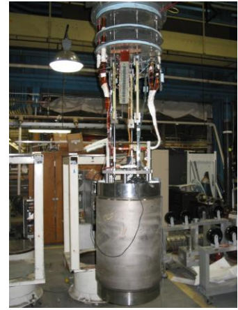
Fig. 29: A 10.2 T Nb 3 Sn dipole designed and built at BNL & tested at the Vertical Test Facility.
