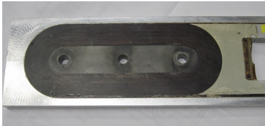
Fig. 25: Sub-scale SM-series test coil (LBNL-type) made at BNL. All coils in the proposed proof-of-principle magnets will be similar to this; two would be almost identical.
