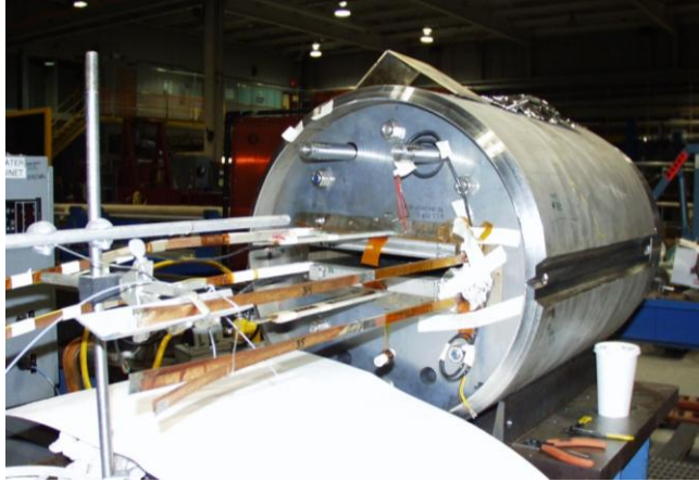
Fig. 29: A 10.2 T Nb 3 Sn dipole designed and built at BNL & tested at the Vertical Test Facility.
