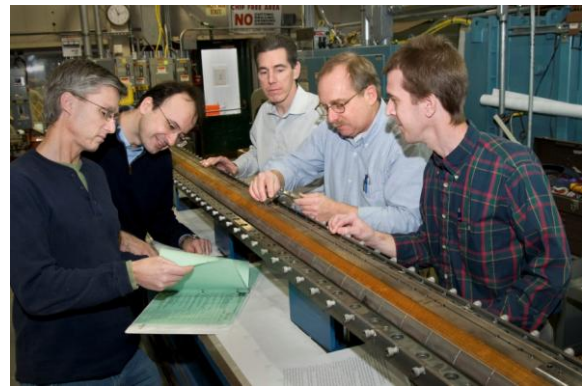
Fig. 30: 3.4-m-long Nb 3 Sn racetrack coil that was wound, cured, reacted and impregnated at BNL. Left: With oven. Right: Being examined by the members of US LARP collaboration.
