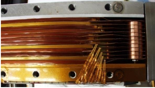
Fig. 6. Left: Heaters between HTS coils. Right: Stable operation at 30 K with 25-W heat load.
