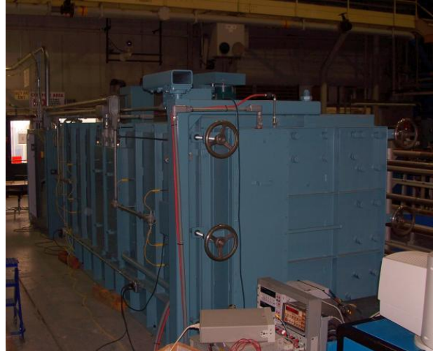
Fig. 27: Ovens for reacting Nb 3 Sn cable and coils. Left: Cubical volume (about 1.1 m 3 ). Right: Oven for long coils (up to 4 meters). Either oven can be used for the PoP coils.
