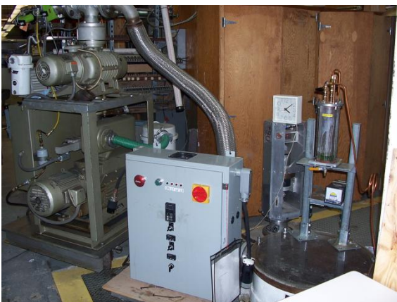
Fig. 28: Vertical and horizontal vacuum impregnation fixtures for impregnating Nb 3 Sn coils; either could be modified for vacuum impregnating Nb 3 Sn coils for the PoP magnet.
