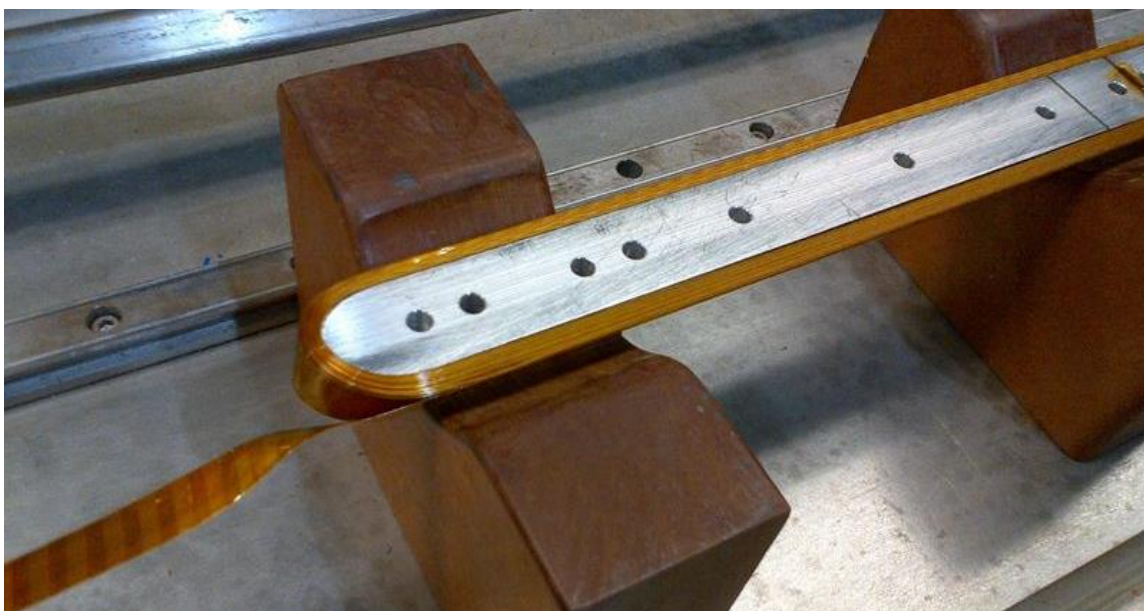
Fig.4. The 20-turn pole winding after fabrication. The 12 mm wide HTS tape conductor with its Kapton CI wrap is visible on the left.
