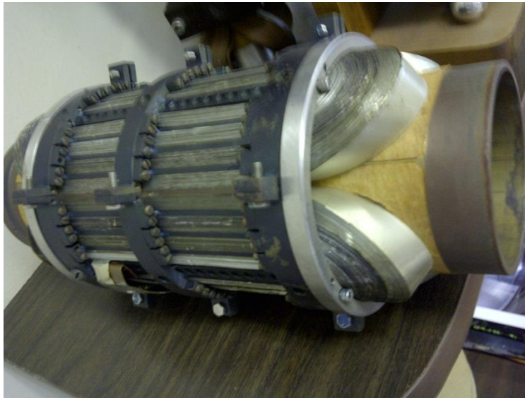
Figure 5. An early \cos \theta coil made with \text{Nb}_3\text{Sn} tape.
