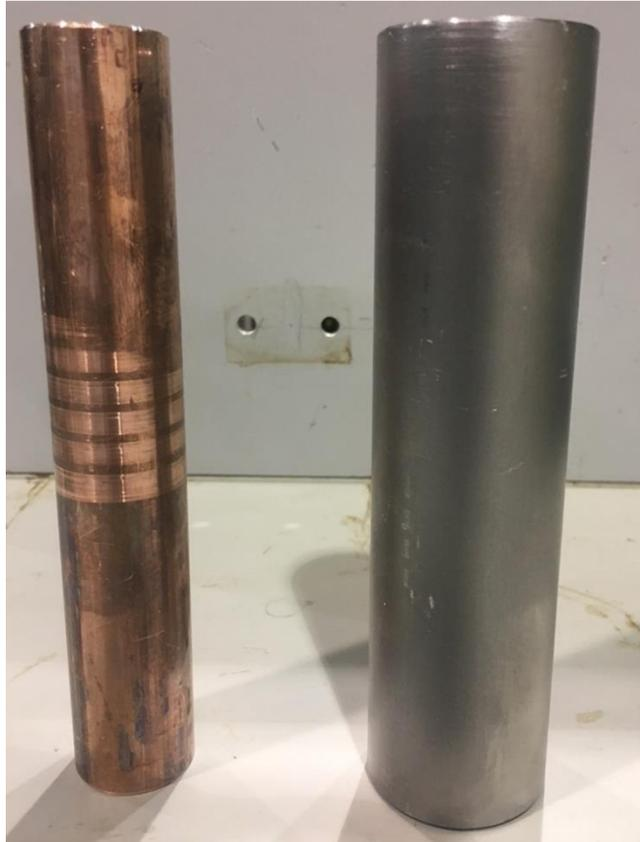
Fig.22. NbTi rods for making LTS shielding tubes provided by Bruker [19] (right) and by Luvata [20] (left).
