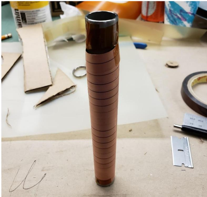
Fig. 24: 12 mm wide HTS tape spirally wrapped around a tube.
