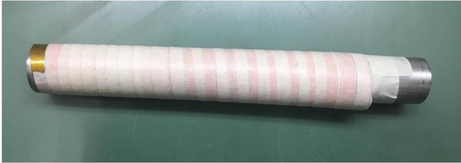
Fig. 25: 12 mm wide HTS tape spirally wrapped around a tube and then further wrapped with insulation to hold it securely.
