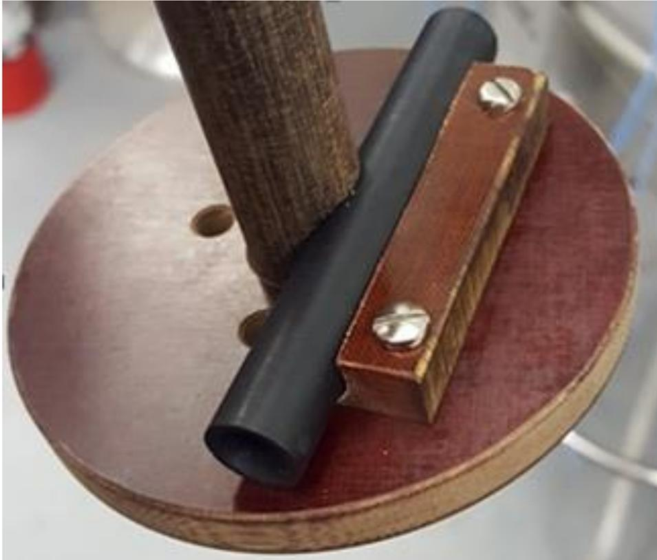
Fig.21. Bi2223 tube provided by CAN superconductor [18]. The tube and test holder will be inserted inside the bore of a coil providing background field.
