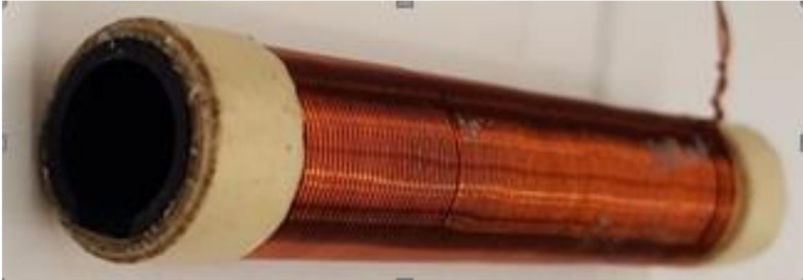
Fig. 30. Copper windings on the HTS tube to immerse it in a field that is primarily axial.
