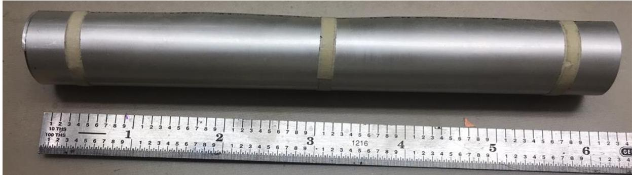
Fig. 28: HTS tape placed on a tube to simulate the shielding test of a primarily dipole field along the beam axis.
