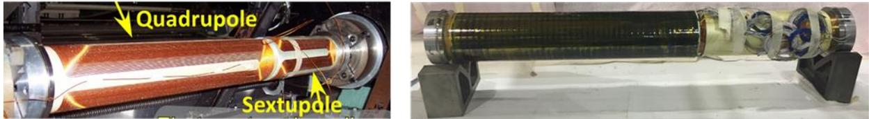
Fig. 40: Superconducting coil windings before (left) and after insulating and structural wrap (right) that will be used in providing the test field in Phase II.
