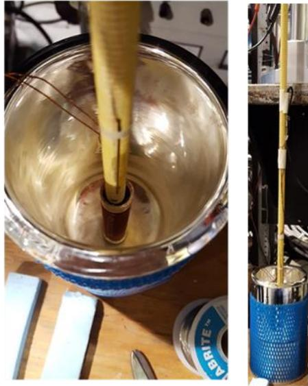
Fig. 32: Bi2223 tube with copper windings on the HTS tube to apply a field that is primarily along the axis placed in the jar that is to be filled with liquid nitrogen with Hall probe placed at the center of the tube.
