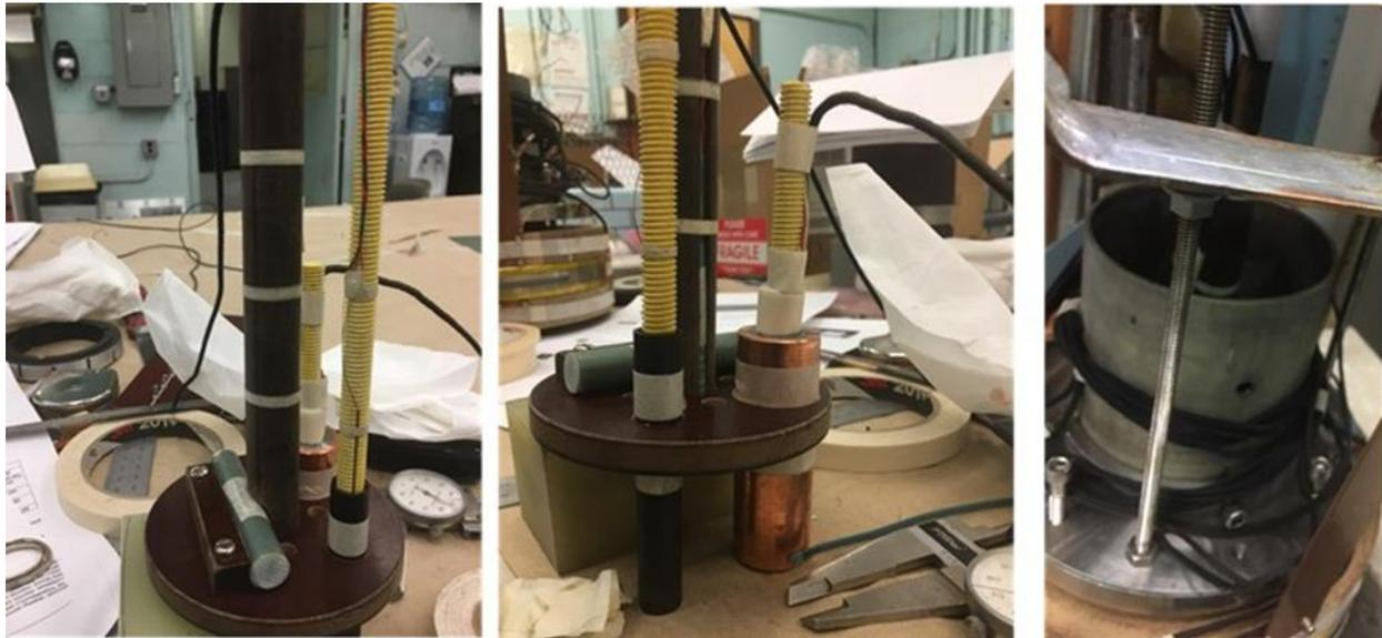
Fig. 34: Pictures on the left and center show the two views of the HTS and LTS tubes and a center tube holding a Hall probe on the axis of the disc. The picture on the right shows the HTS and LTS shielding tubes inside an HTS coil with several Hall probes.
