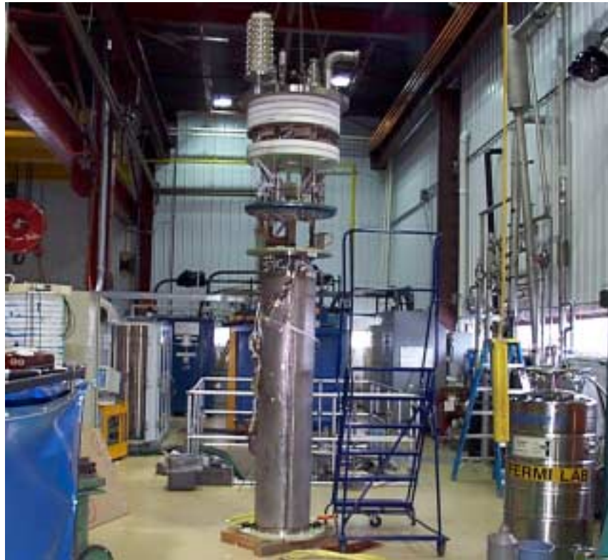
Figure 10.2. The Vertical Magnet Test Facility with a model LHC IR quadrupole ready to be inserted for testing.
