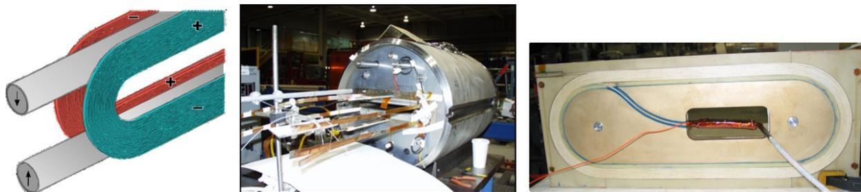
*Fig. 6. Left: Basic design of 2-in-1 common coil dipole, Middle: Nb<sub>3</sub>Sn common coil dipole DCC017 with large open space, Right: An HTS coil, such as a Bi2212 coil that reached 4.3 kA, in a background field.*
