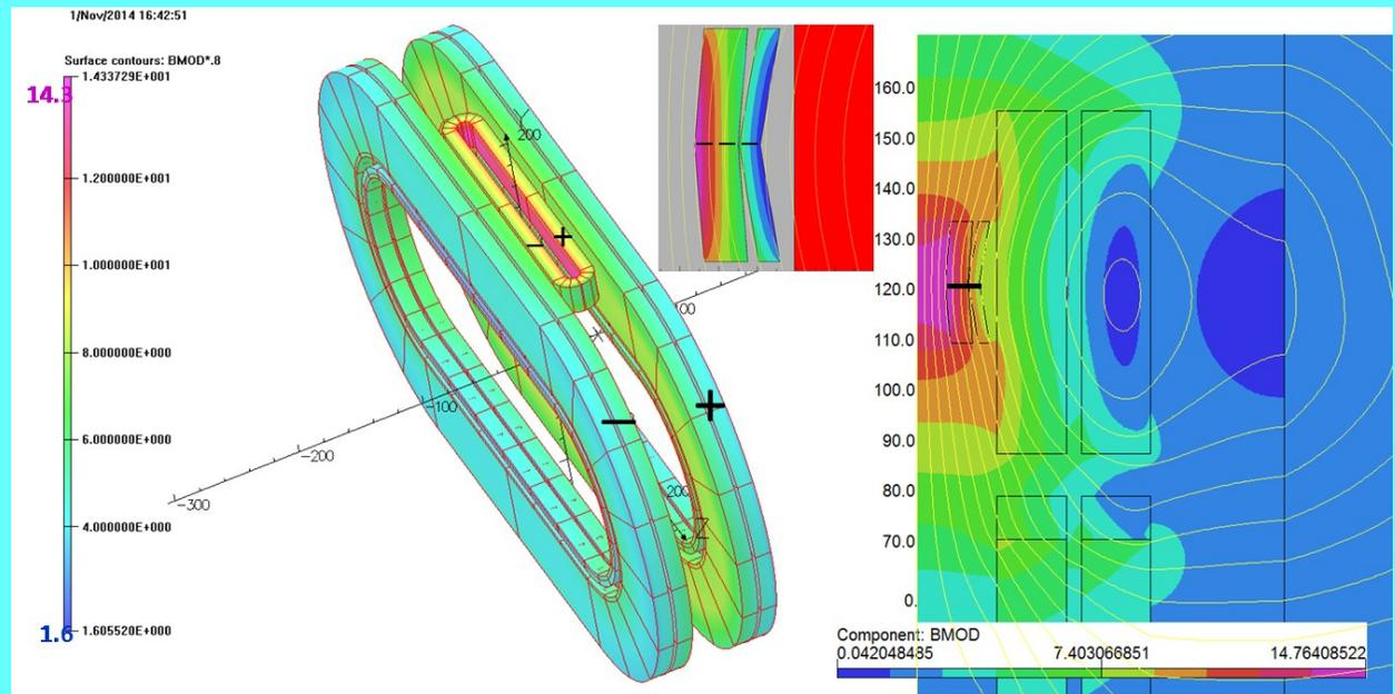
**Fig. 12:** Magnetic model of the Proof-of-Principle configuration to experimentally test the applicability of the proposed technique. A small HTS coil is placed inside the large Nb<sub>3</sub>Sn coil of DCC017. A 2-d model shows that the field lines (yellow) are reasonably aligned parallel to the wide face of the HTS tape. This alignment can be seen more clearly in the inset where field contour is superimposed only on the HTS coils.
