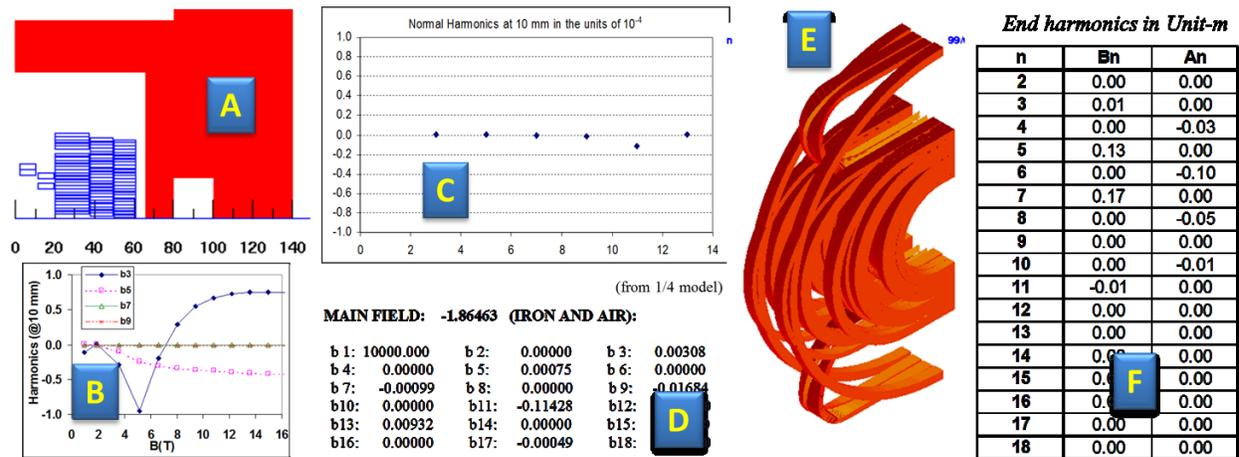
**Fig. 8:** Example of the optimization for good field quality in a common coil design (coil aperture 40 mm, reference radius 10 mm). (a) 1/4 of magnet cross section in one aperture, (b) normal saturation induced-harmonics, (c) plot of geometric harmonics, (d) values of geometric harmonics, (e) optimized end geometry, and (f) end harmonics.
