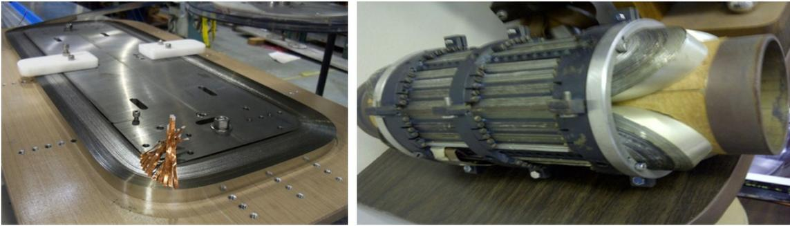
**Fig. 9.** Magnets made with tape conductors. On the left is a recently made FRIB coil using ReBCO tape, and on the right are four coils made using Nb3Sn tape and assembled in a quadrupole configuration in the 1960's.
