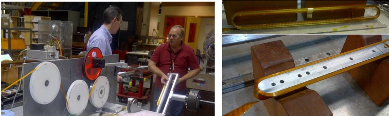
**Fig.3.** Left: Coil with Kapton-insulated HTS tape being wound on the fixture. Right: Wound and fully cured HTS coil (top-right shows stand-alone block and bottom-right shows with pole spacer).
