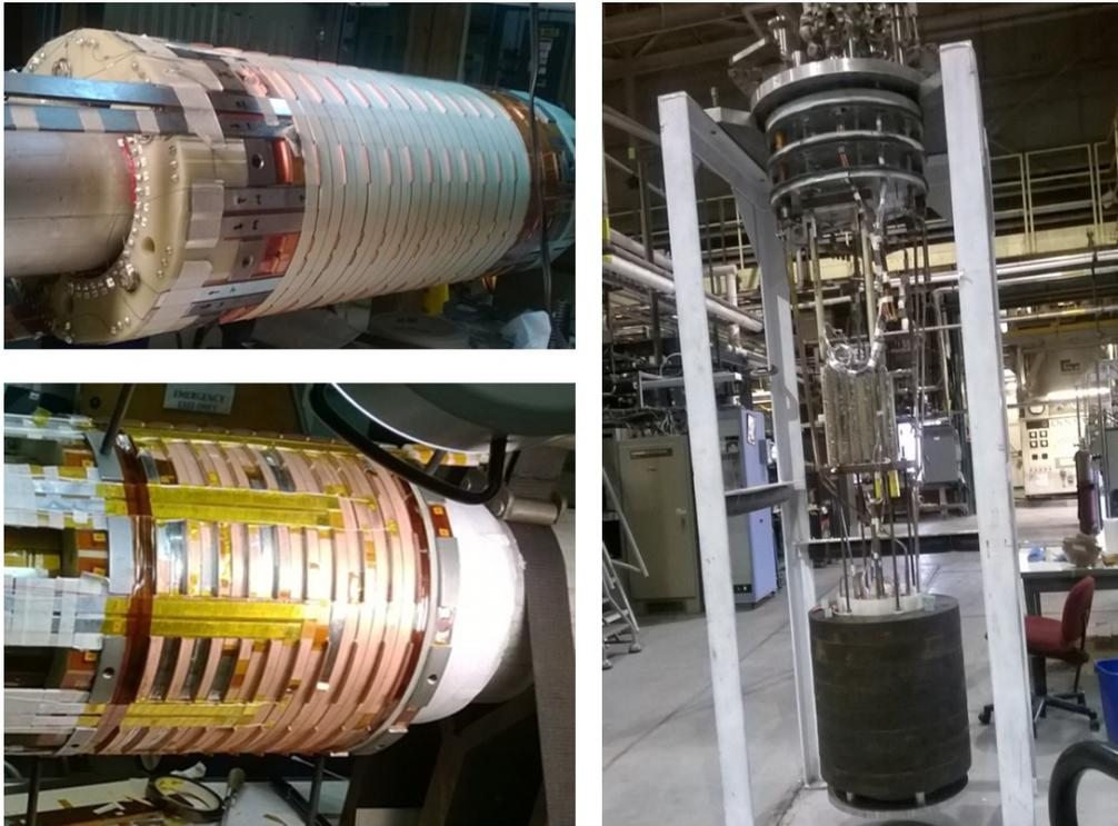
*Fig. 4. High Field HTS SMES magnet with inner coil at top-left, outer coil at bottom-left and fully assembled magnet on test stand at right.*
