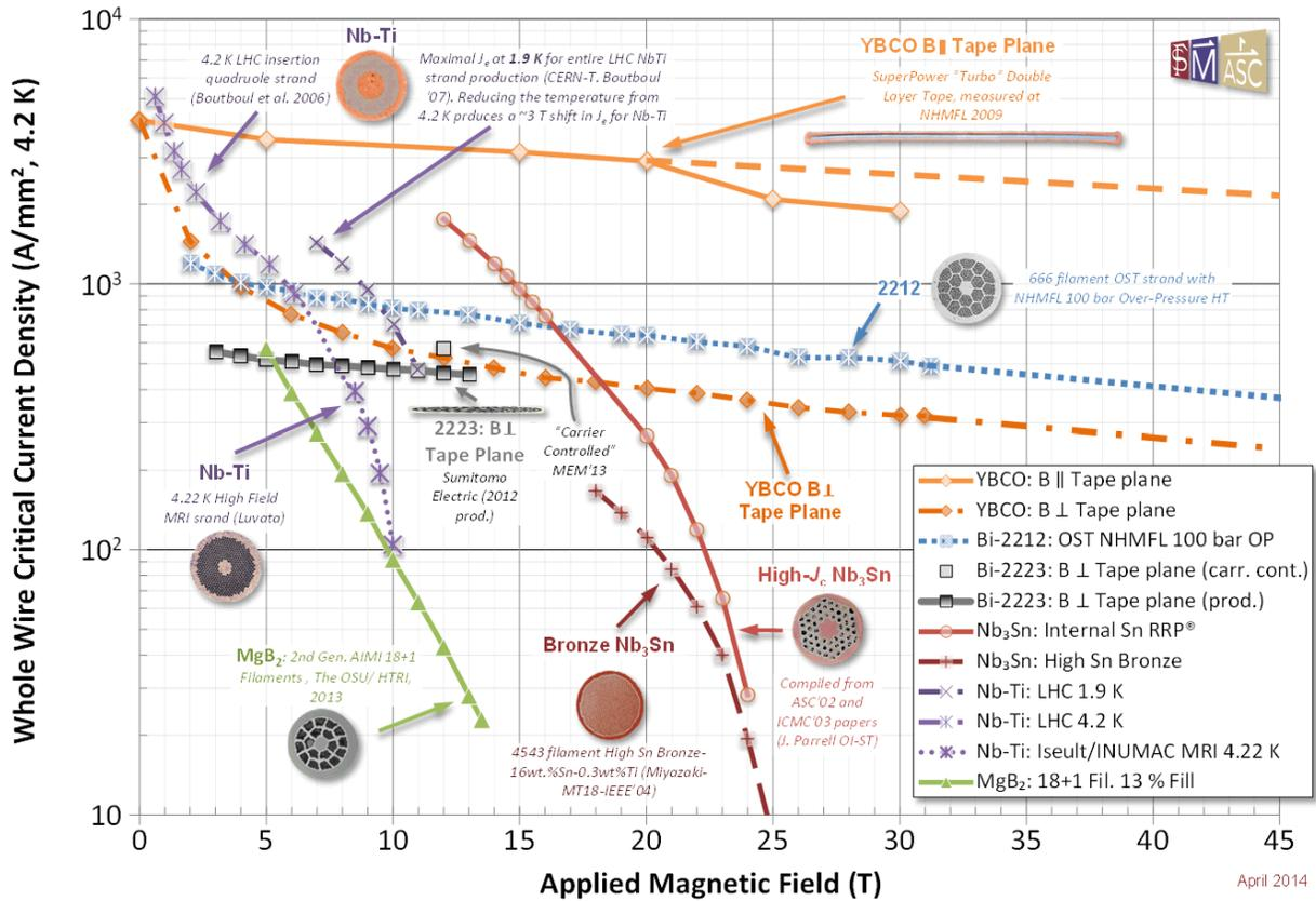
*Fig.1. Engineering current density for HTS (YBCO tape and Bi2212 wire) compared to other high field superconductors, showing the advantages of HTS at high fields. Data compiled by P. Lee, NHMFL.*
