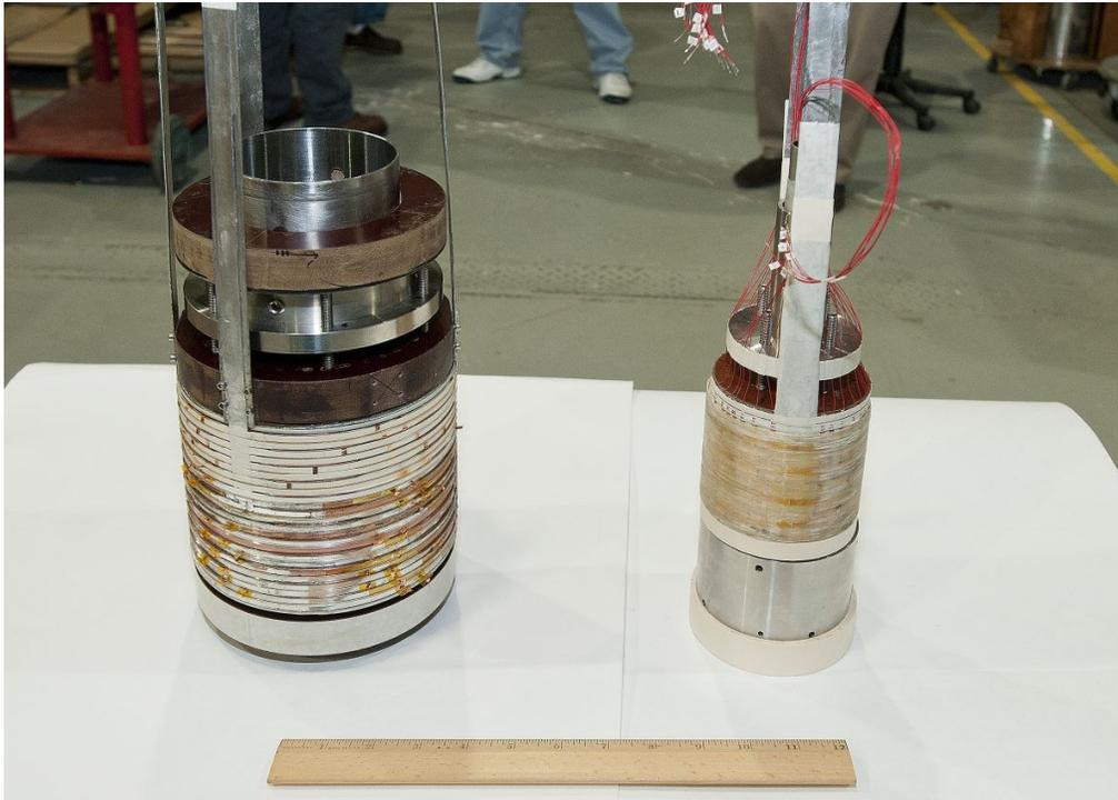
**Fig. 2.** Left: 100 mm bore “midsert” solenoid of 24 YBCO pancakes. Right: 25 mm 14-pancake YBCO “insert” magnet. Half-length “midsert” solenoid of 12 YBCO pancakes generated a maximum ambient (peak) field of  $\sim 9.2$  T at 4 K and full-length 14-pancake YBCO “insert” magnet that generated nearly 16 T on axis (a record for HTS). The two are designed to generate a total field of over 22 T.
