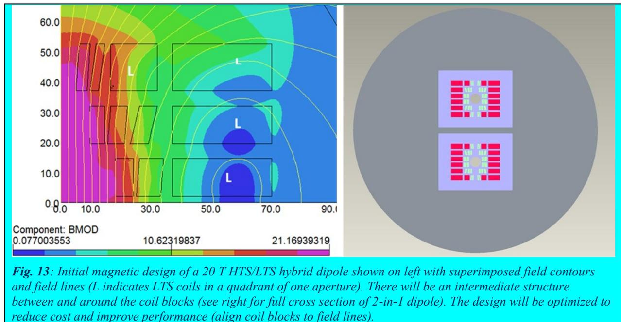
**Fig. 13:** Initial magnetic design of a 20 T HTS/LTS hybrid dipole shown on left with superimposed field contours and field lines (L indicates LTS coils in a quadrant of one aperture). There will be an intermediate structure between and around the coil blocks (see right for full cross section of 2-in-1 dipole). The design will be optimized to reduce cost and improve performance (align coil blocks to field lines).
