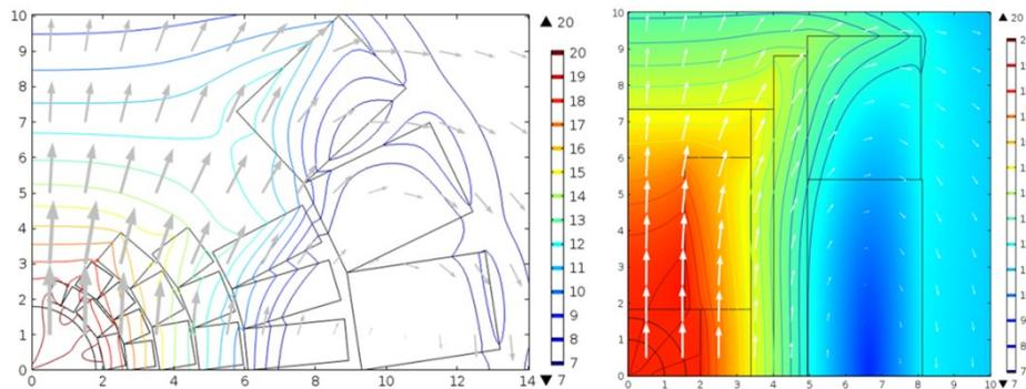
**Fig. 10:** Cosine theta hybrid design (left) and block coil hybrid design (right) evaluated during Phase I. The block coil is preferred for separating HTS/LTS coil layers and for better optimization.
