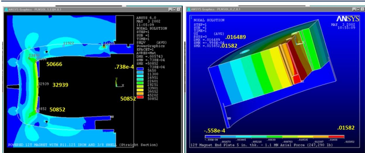
**Fig. 7.** ANSYS simulation showing stresses in the collar (left) and on the end plates (right) in the common coil dipole DCC017.
