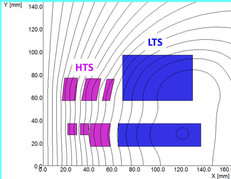
**Fig. 11:** Optimized design to significantly reduce magnetization-induced errors. The 12 mm wide conductor makes six LTS and four HTS layers with the wide side of the HTS tape generally aligned to the field lines.
