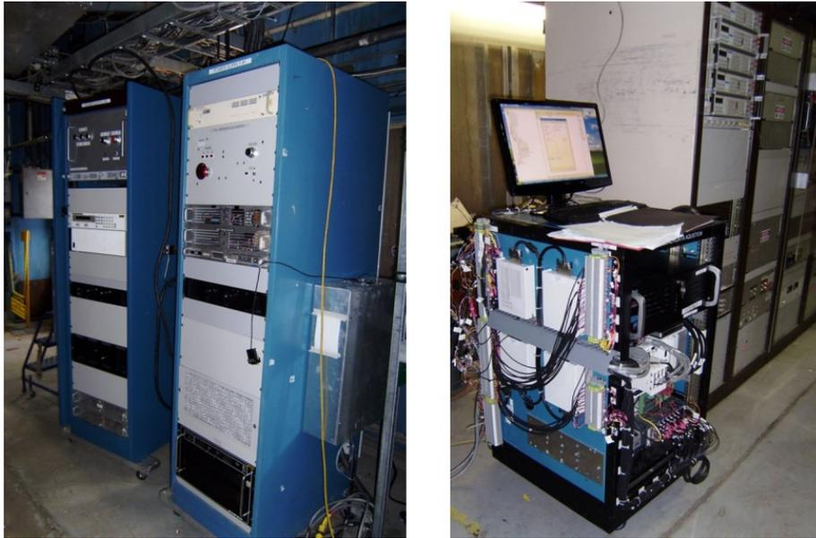
*Fig. 5. Advanced quench protection system (patent awarded) that can isolate pre-quench voltage below 1 mV and can tolerate isolation voltage. This is a key component of the HTS technology program.*
