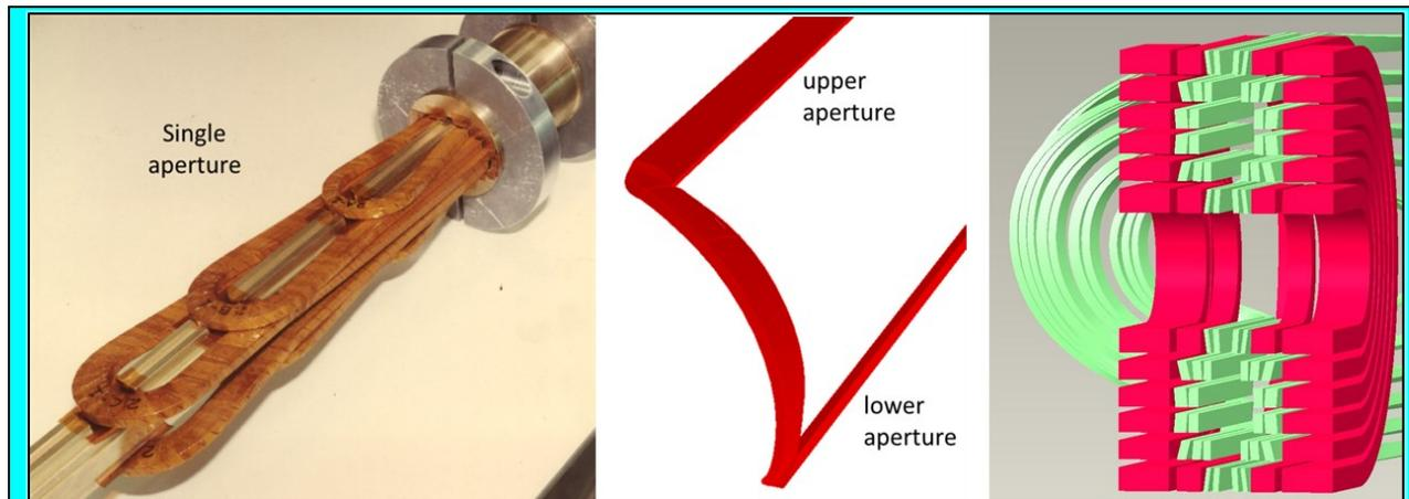
**Fig. 14:** Vertically lifted coil ends for a single aperture dipole (see left) and a horizontally lifted ends for a 2-in-1 common coil design (see right). Only the blocks needed to clear the aperture would be lifted vertically or sideways. One sideways lifted block is shown more clearly in the figure on the middle.
