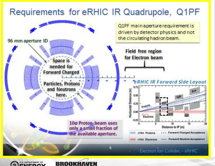
We will use the recent Q1PF quadrupole coil crosssection for investigation. We will study the superconducting shielding with and inside the iron yoke as an alternate to the active field cancelling external coils.
