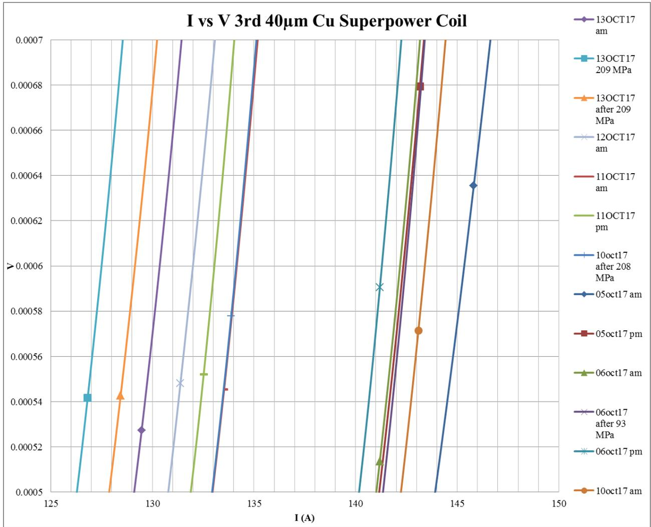
**Figure 31:** *I vs V for 3rd 40µm Coil throughout its test time*
