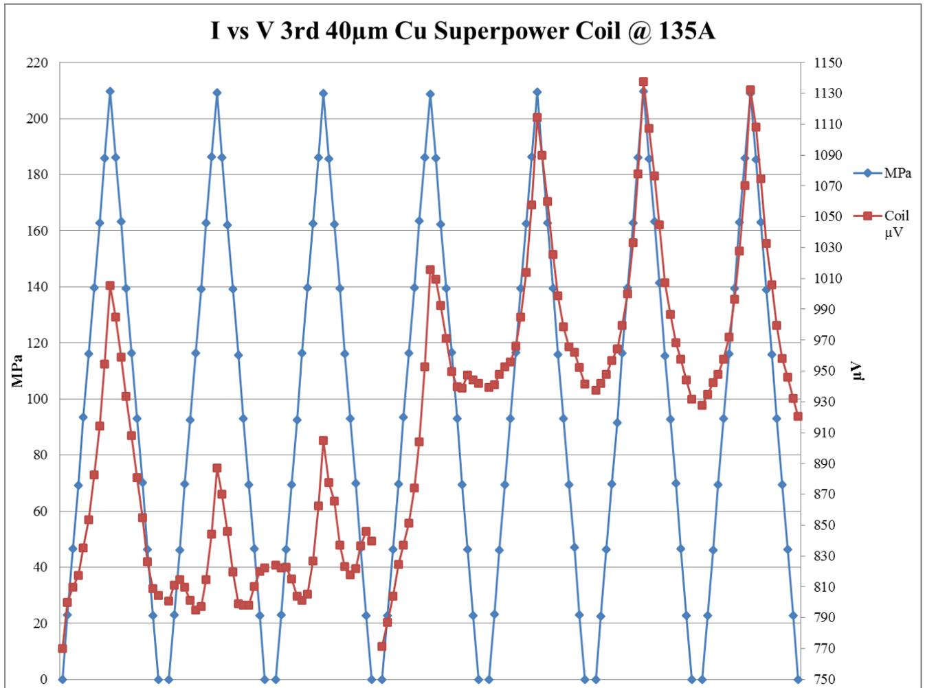
**Figure 35:** 3rd 40µm Coil compression behavior at 135 A
