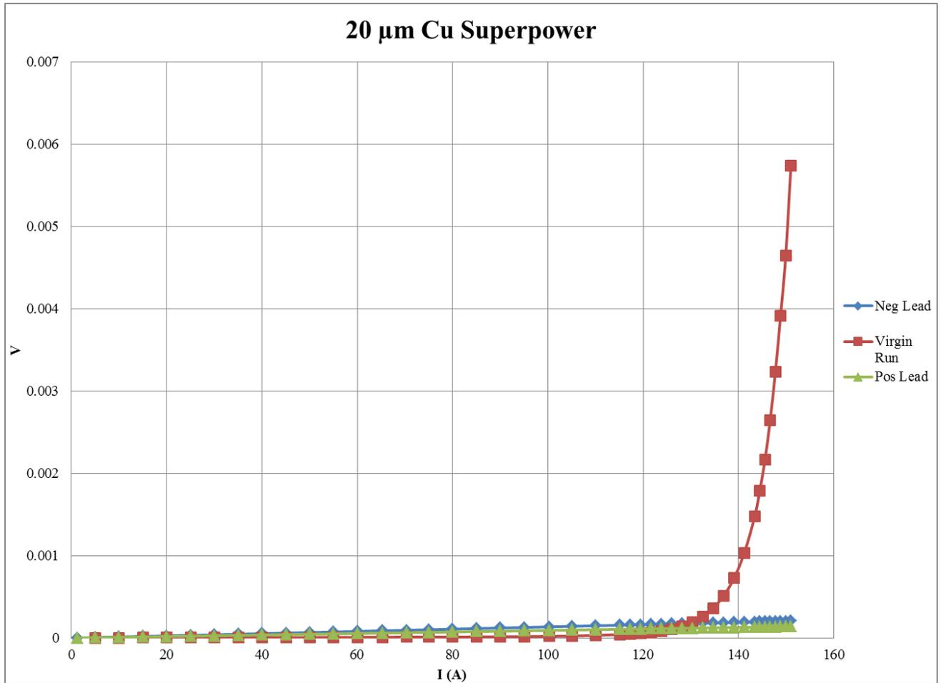
**Figure 46:** Initial I vs V for 20 $\mu\text{m}$  Coil
