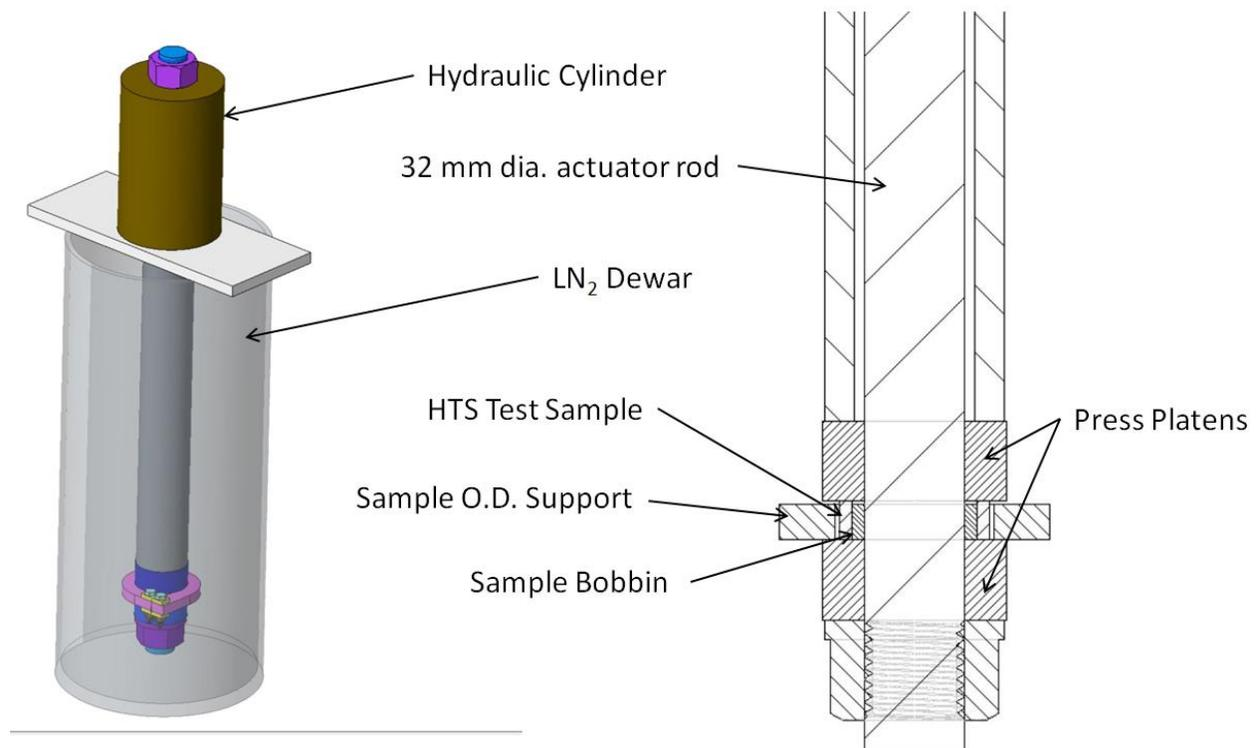
*Figure 3: CAD rendering of the compression fixture*
