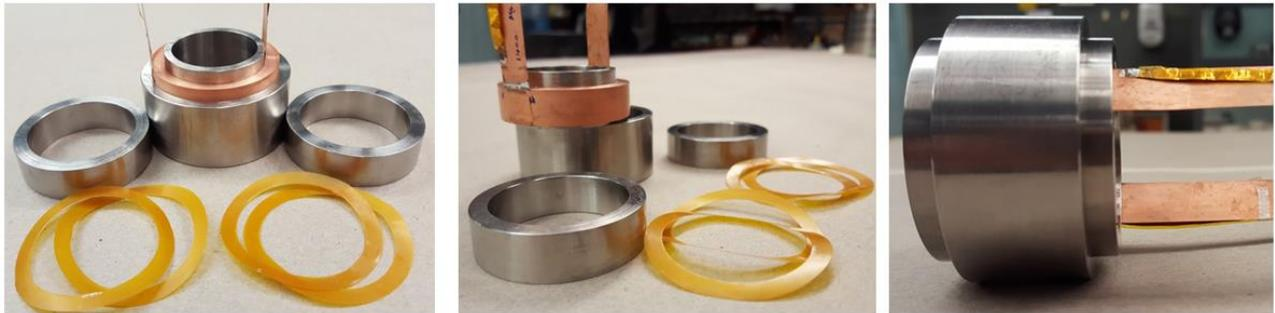
**Figure 14:** Similar to description in figure 12, except, replaced 5 mil Mylar caps with two 5 mil Nomex (softer insulator) caps on top and bottom of coil
