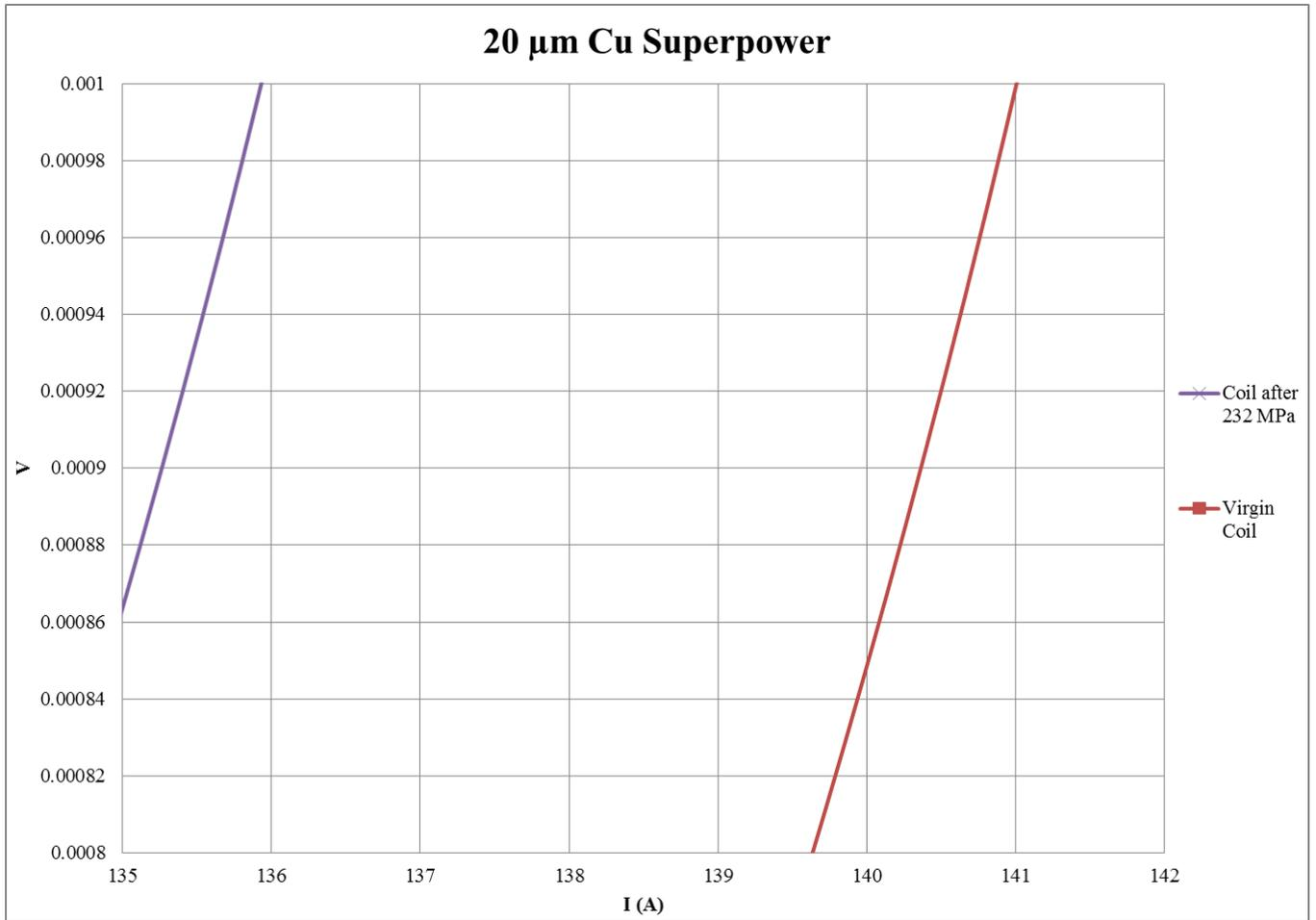
**Figure 53:** *I vs V for 20μm Coil*
