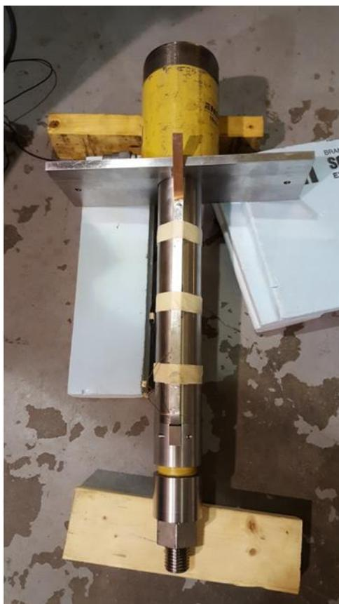
*Figure 7: Compression fixture with SuperPower 2G HTS 65 $\mu$ m Cu coil in Kevlar and Epoxy Wrapping*
