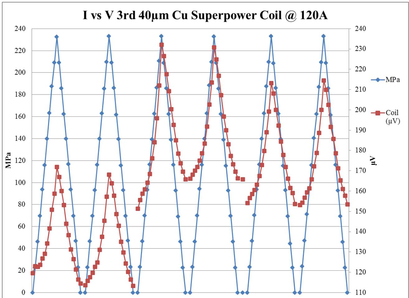
**Figure 39:** 3rd 40µm Coil compression behavior at 120 A
