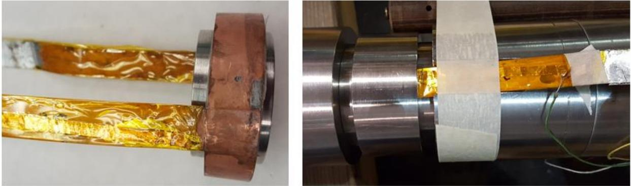
**Figure 13:** In addition to the description in figure 11, added insulated lead voltage taps for more accurate data
