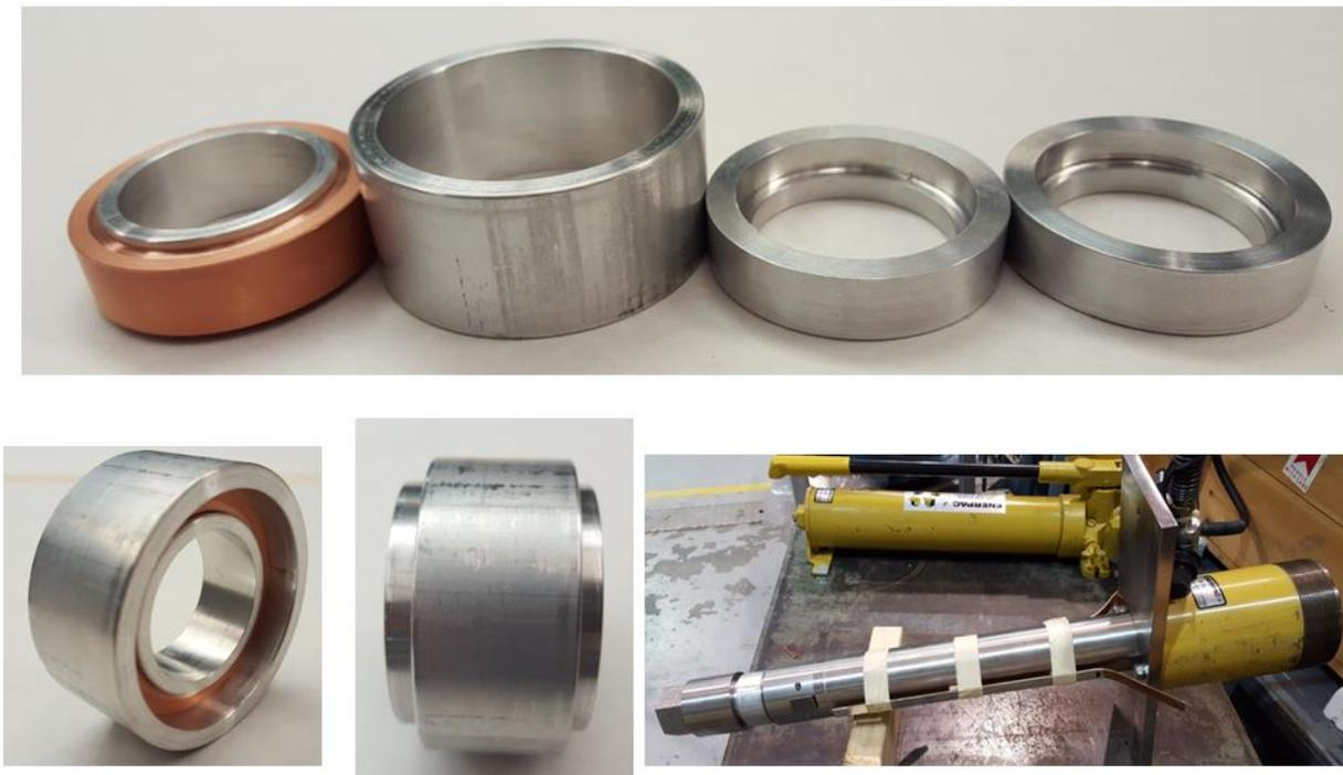
**Figure 10:** Aluminum outer ring and double piston – improved design; however, Aluminum warped under compressive pressures in excess of 140 MPa
