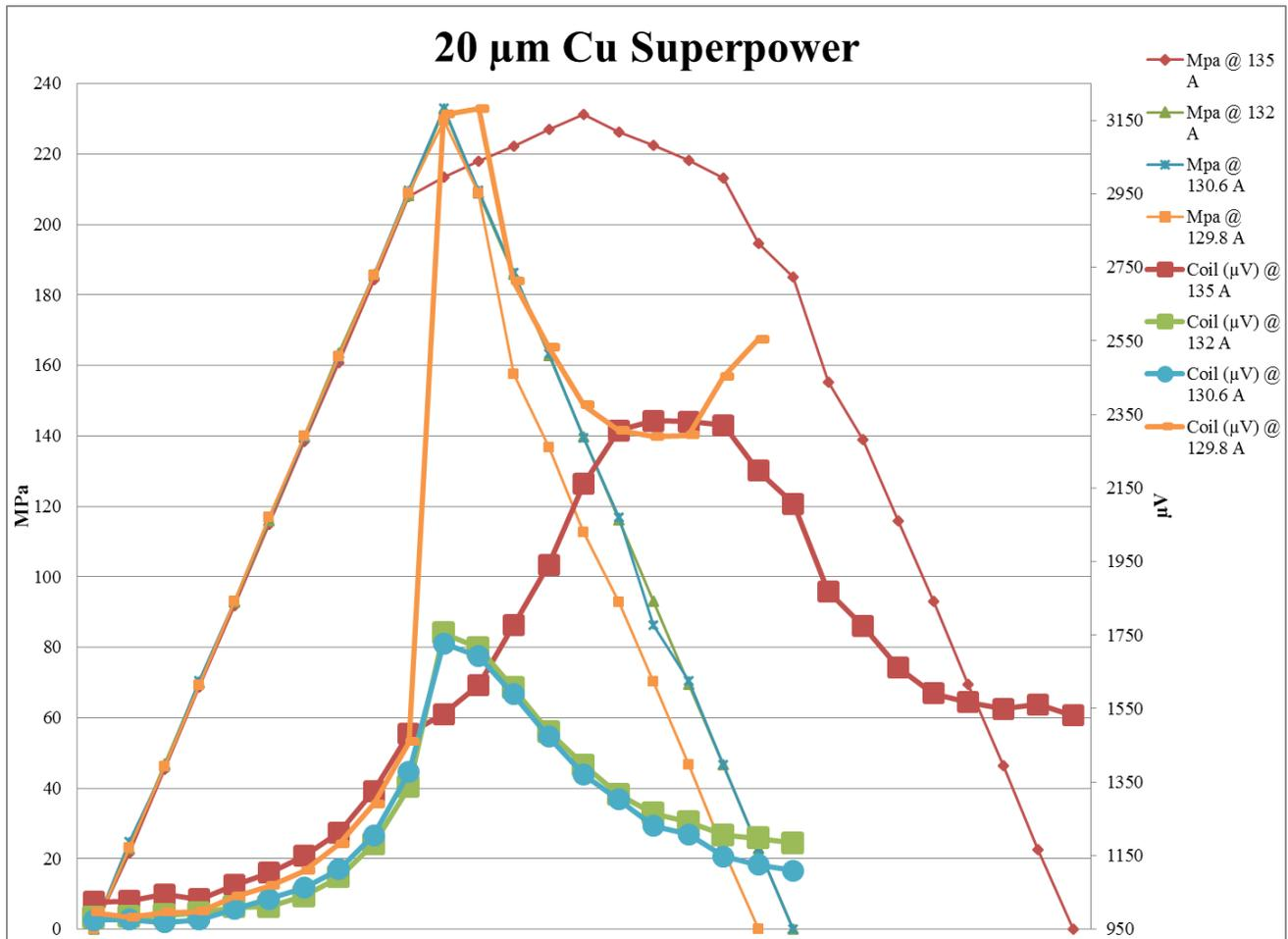
**Figure 57:** 20 $\mu$ m Coil compression behavior at various currents; each cycle starting around 1000 $\mu$ V
