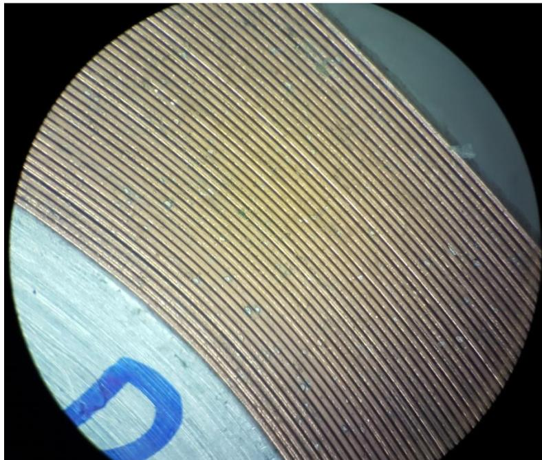
*Picture 2: Bottom of the coil after 25 MPa of compressive loading under a microscope*
