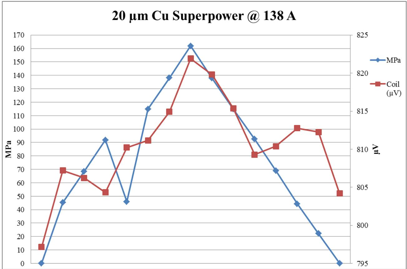
Figure 48: 20μm Coil compression behavior at 138 A
