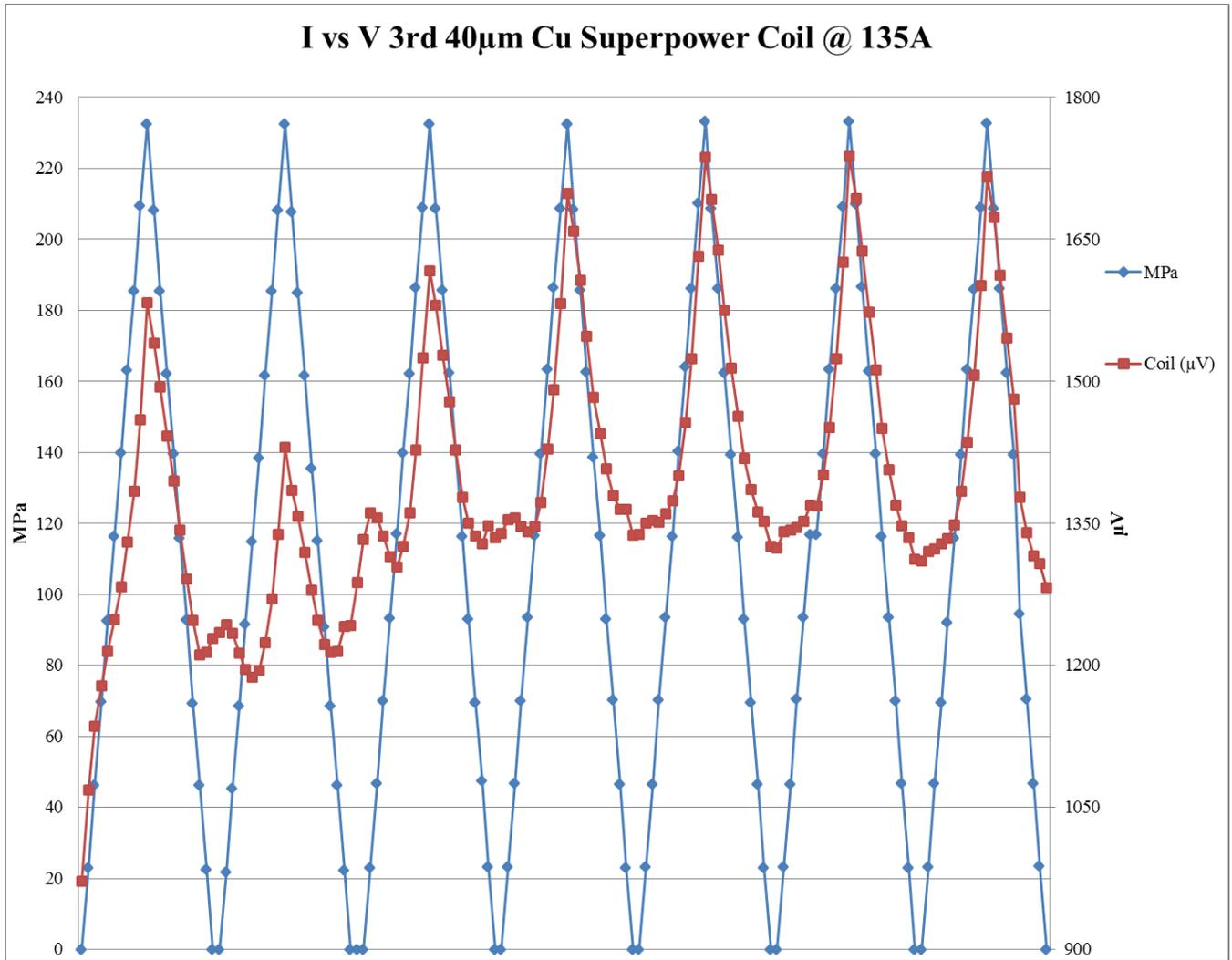
**Figure 37:** 3rd 40µm Coil compression behavior at 135 A
