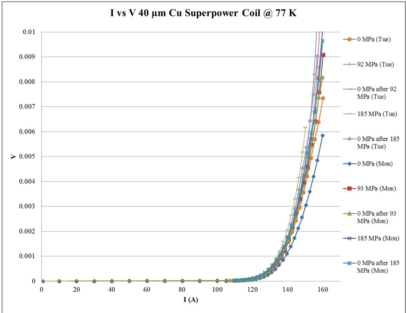
**Figure 23:** *I vs V for 2nd 40 $\mu$ m Coil @ 77K*
