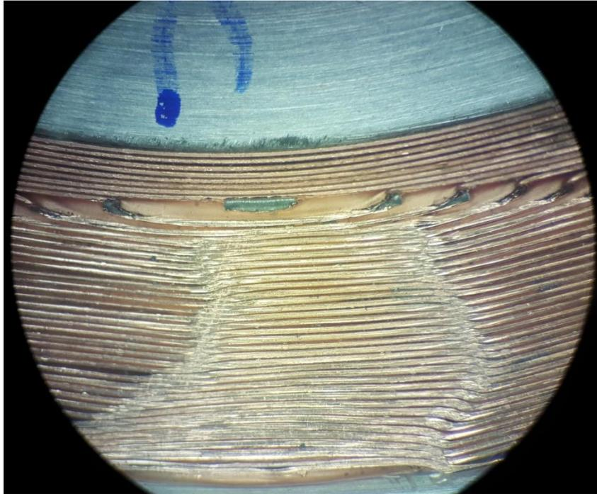
**Picture 5:** *Top of the coil after 175 MPa of compressive loading under a microscope*
