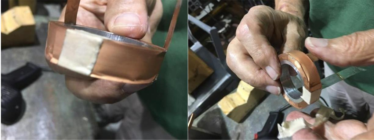
**Figure 17:** Physical deformation in 43 turn coil after compression cycles
