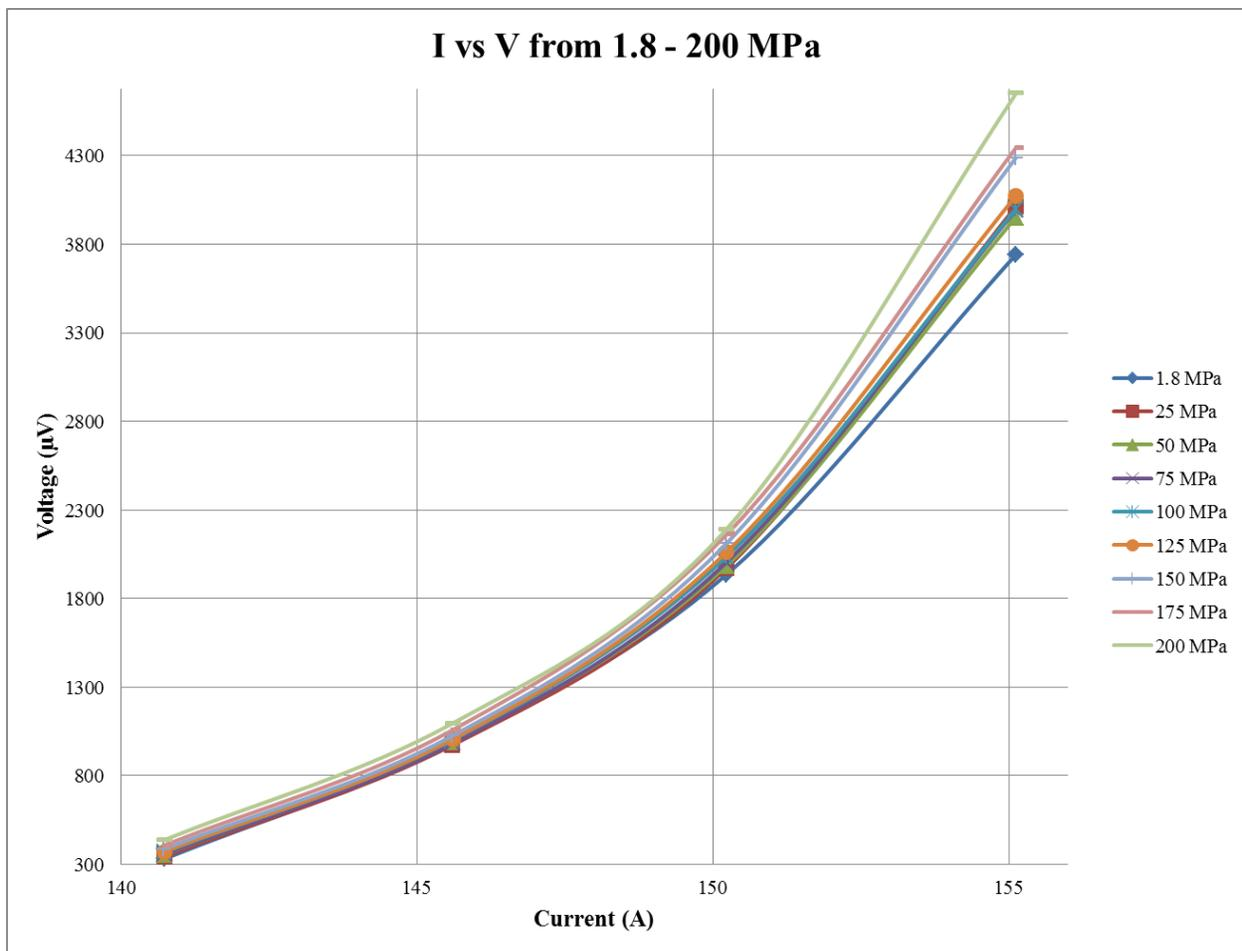
**Figure 15:** I vs V for SuperPower 2G HTS 65 $\mu$ m Cu coil in Kevlar and Epoxy Wrapping at various compressive pressures
