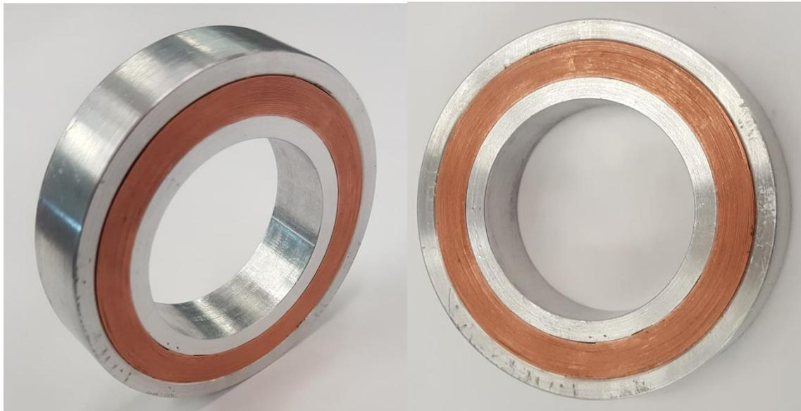
**Figure 18:** Second, 41 turn, SuperPower 2G HTS 65 $\mu\text{m}$  Cu coil in Aluminum outer ring
