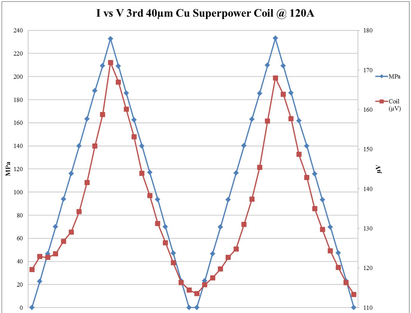
Figure 38: 3rd 40µm Coil compression behavior at 120 A
