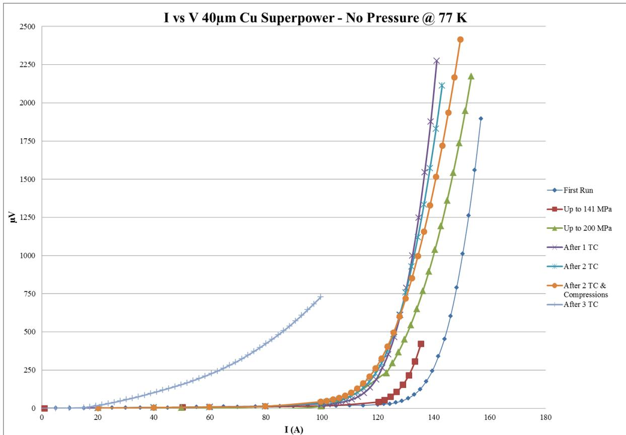
**Figure 20:** *I vs V for 40 $\mu\text{m}$  Coil through multiple compressive and thermal cycles*
