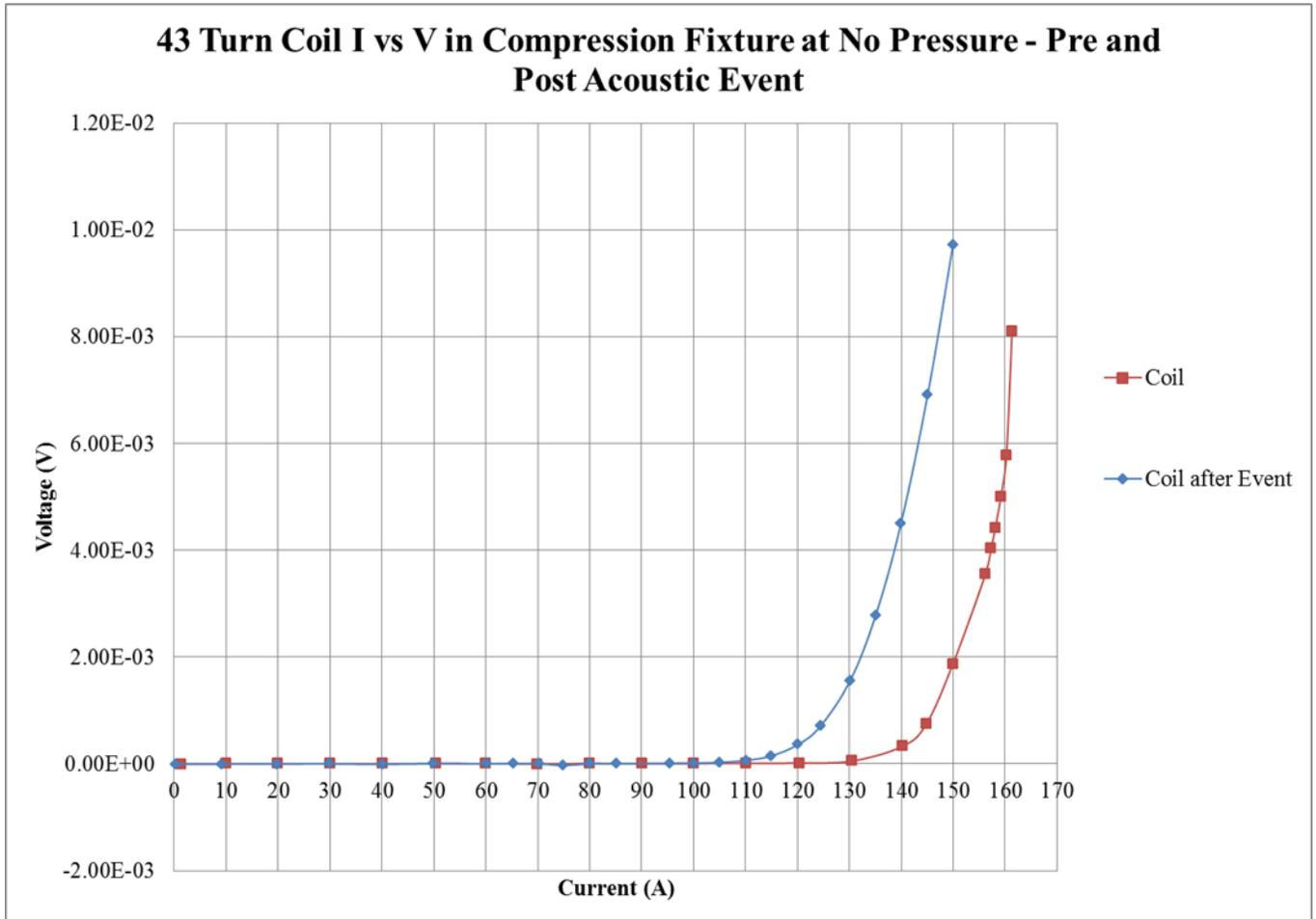
**Figure 16:** I vs V for SuperPower 2G HTS 65 $\mu$ m Cu coil in Kevlar and Epoxy Wrapping before and after acoustic event
