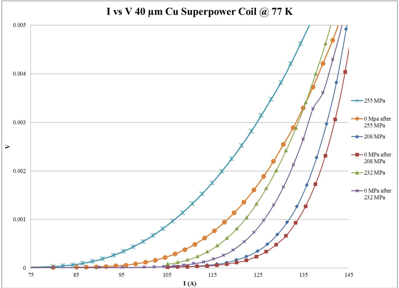
**Figure 29:** *I vs V for 2nd 40μm Coil with and without compressive pressure*
