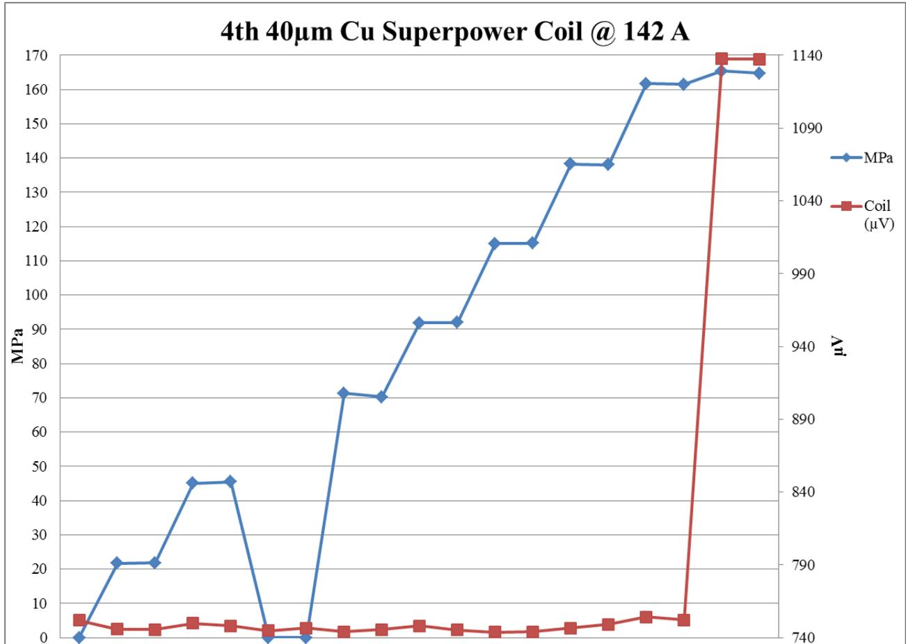
Figure 41: 4th 40 $\mu\text{m}$  Coil compression behavior at 142 A
