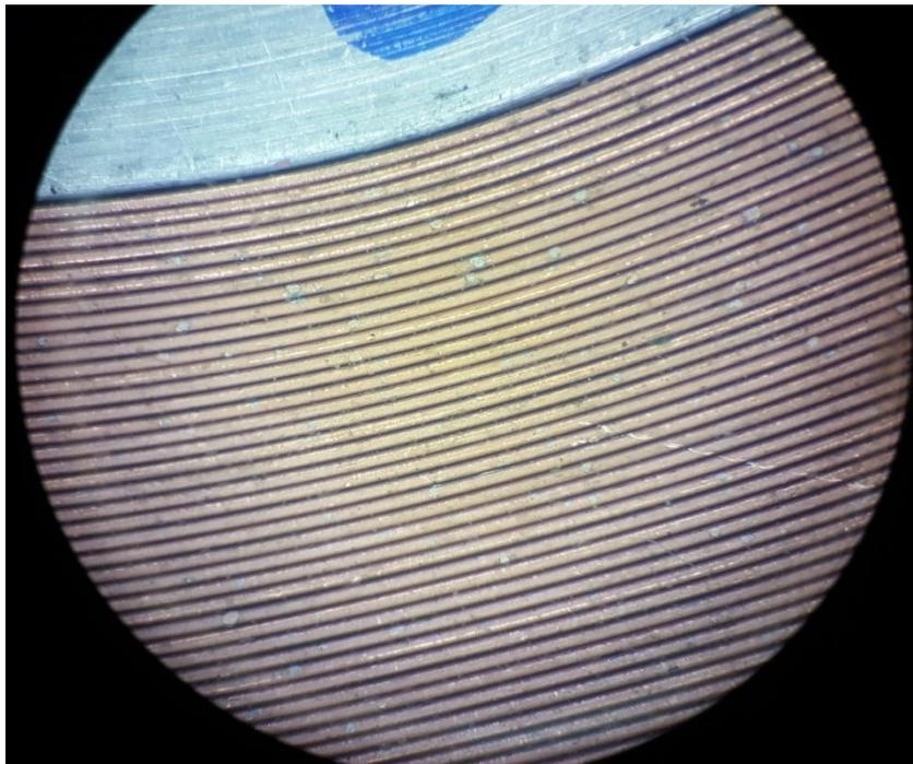
**Picture 4:** *Bottom of the coil after 100 MPa of compressive loading under a microscope*
