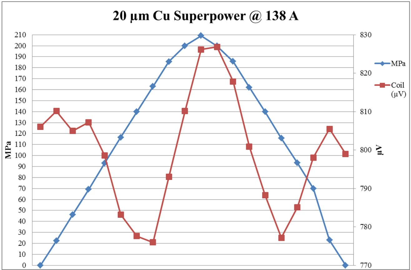
Figure 50: 20μm Coil compression behavior at 138 A
