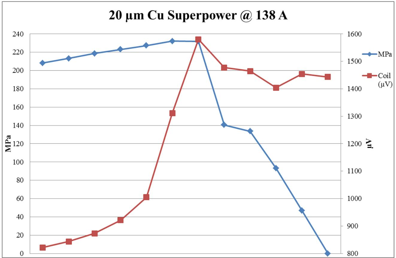
**Figure 51:** 20μm Coil compression behavior at 138 A
