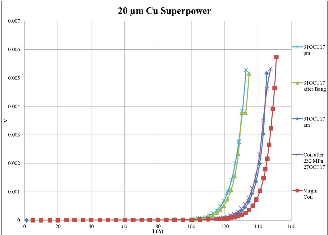
Figure 61: I vs V for 20μm Coil
