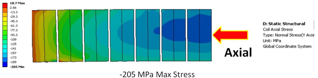
**Figure 2:** ANSYS FE simulation of orthogonal stress on coils in the axial direction at 4K & 25T
