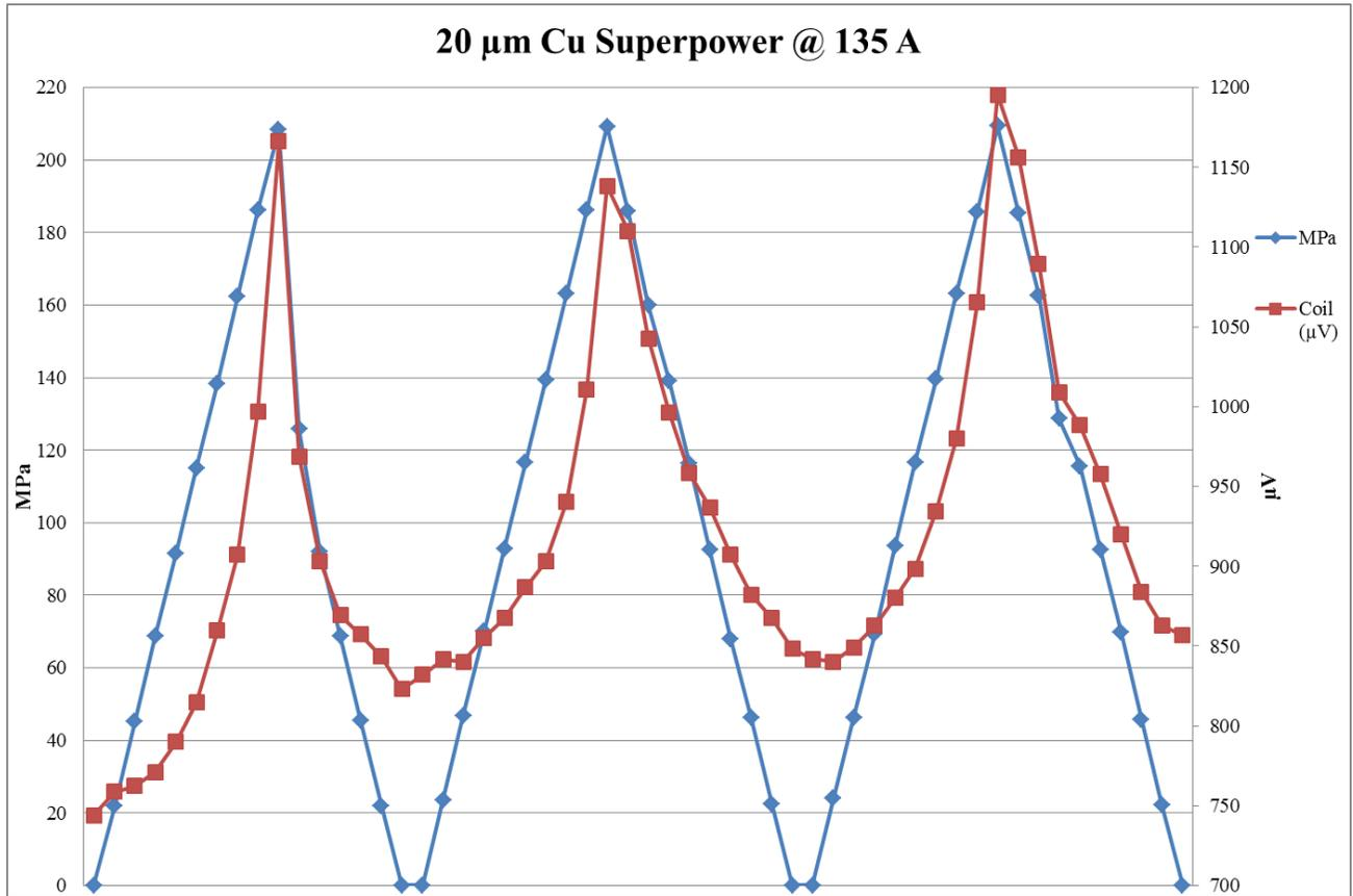
Figure 56: 20μm Coil compression behavior at 135 A
