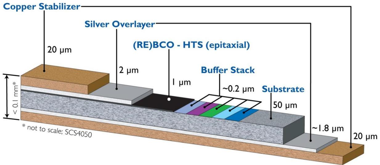
**Figure 1:** SuperPower 2G HTS 40 micron Copper conductor tape architecture<sup>3</sup>
