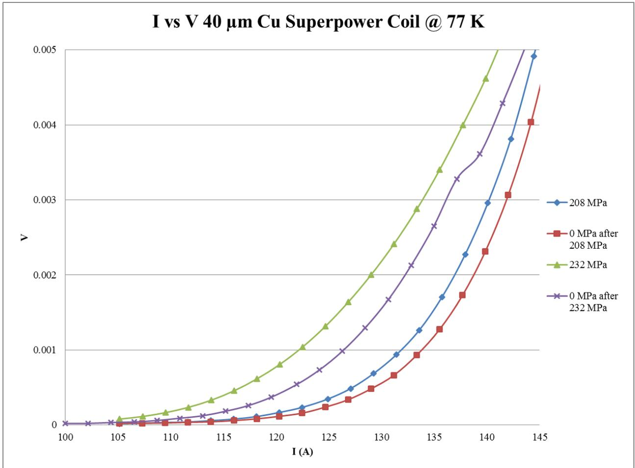
**Figure 27:** *I vs V for 2nd 40μm Coil with and without compressive pressure*
