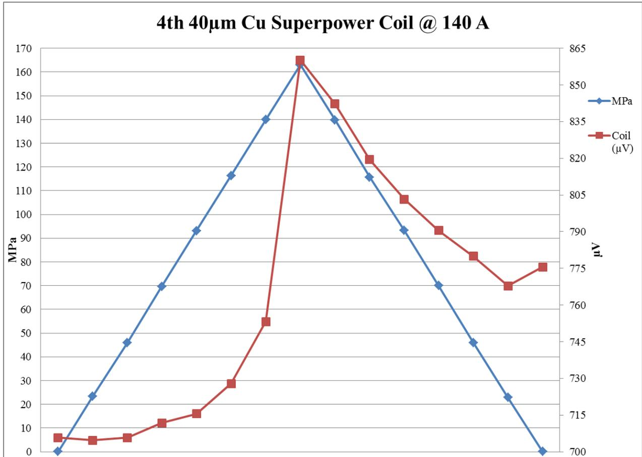
Figure 43: 4th 40µm Coil compression behavior at 140 A
