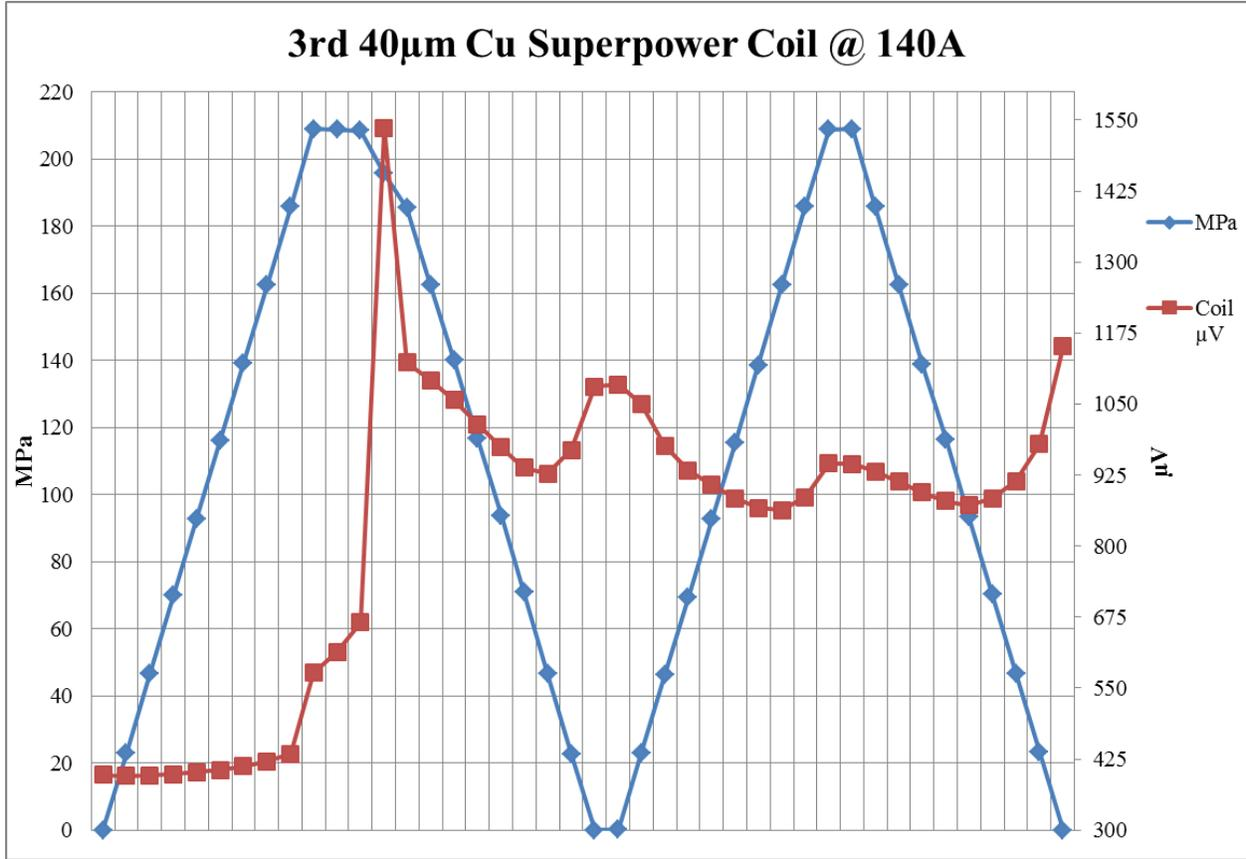
Figure 33: 3rd 40µm Coil compression behavior at 140 A
