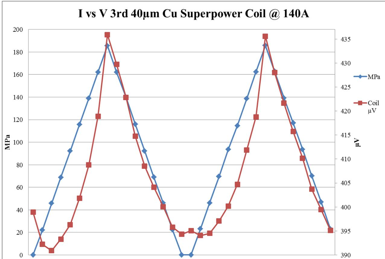
Figure 32: 3rd 40 $\mu\text{m}$  Coil compression behavior at 140 A
