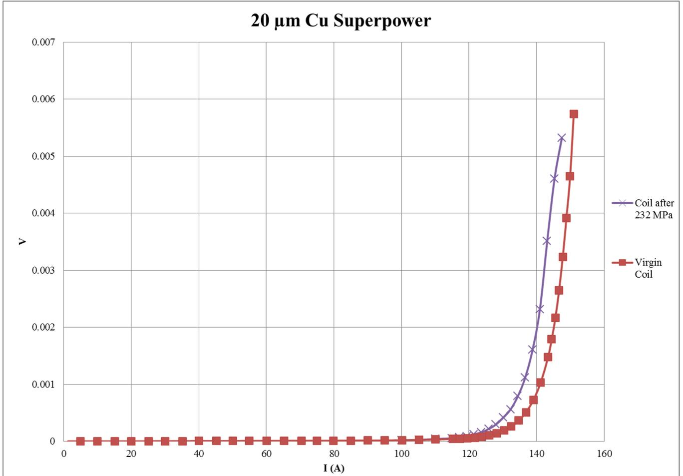
Figure 52: I vs V for 20μm Coil
