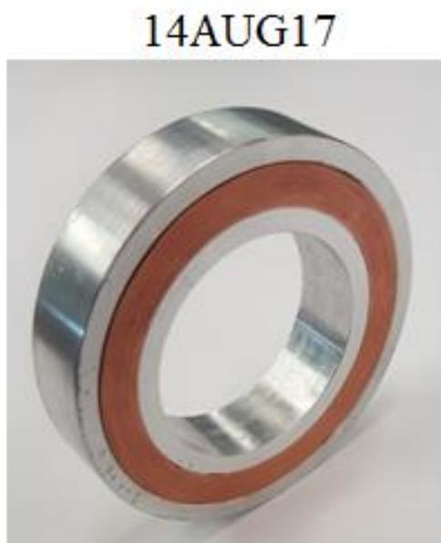
*Figure 8: Aluminum outer ring – did not allow proper compression force distribution across sample*
