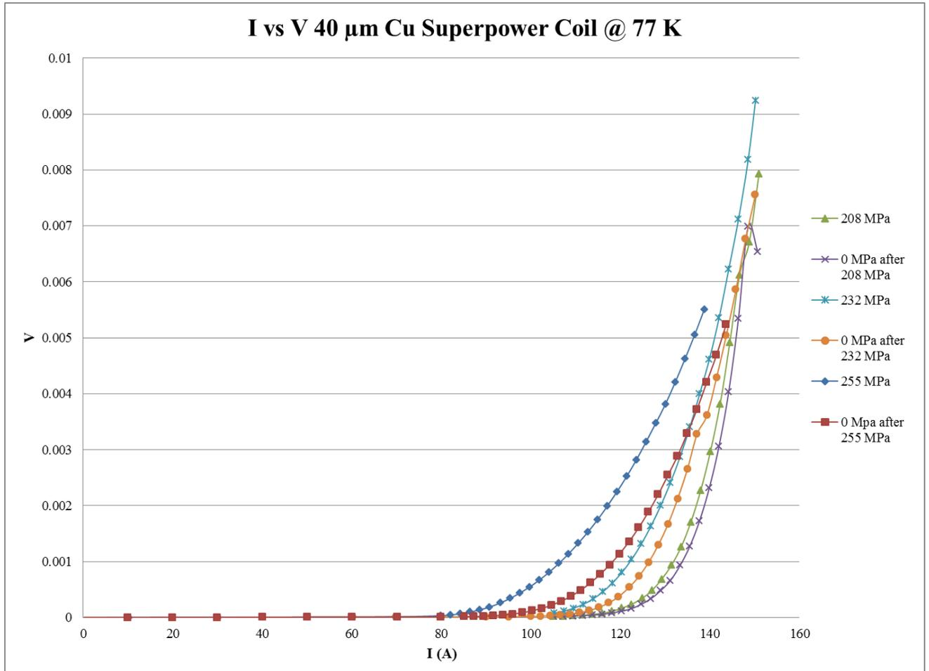
Figure 28: I vs V for 2nd 40μm Coil with and without compressive pressure
