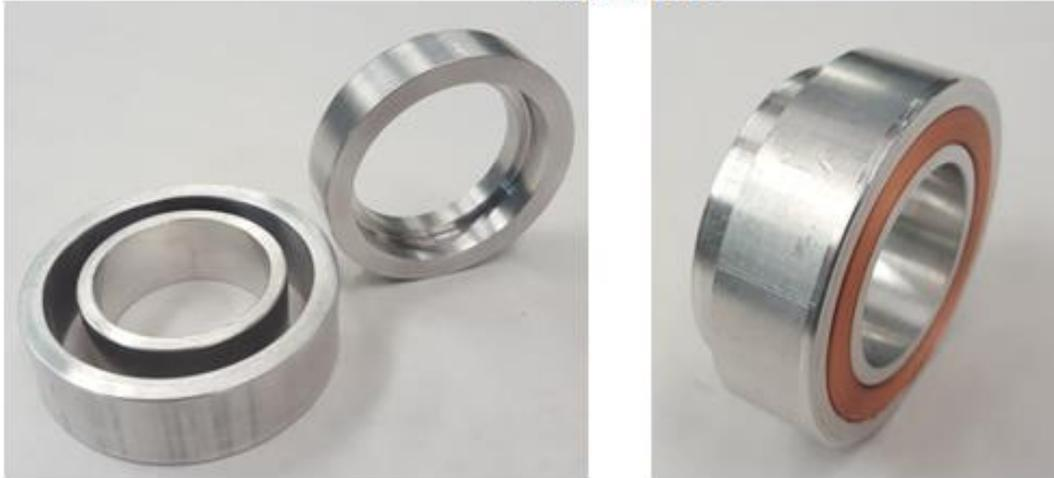
**Figure 9:** Aluminum outer ring and single piston – left void at bottom of sample leading to improper compression force distribution
