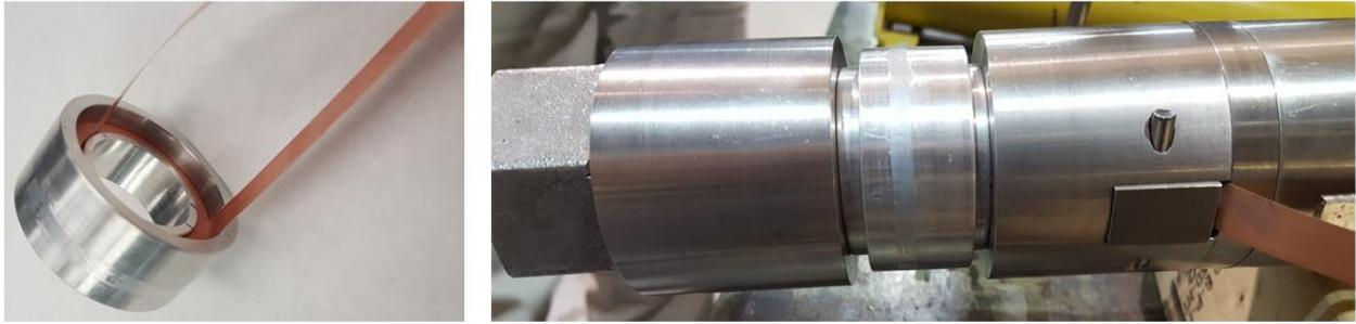
**Figure 11:** *Stainless Steel outer ring and double piston – optimal design*
