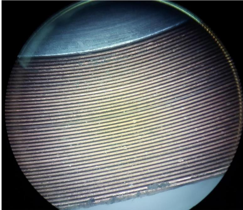
*Picture 1: Top of the coil after 25 MPa of compressive loading under a microscope*
