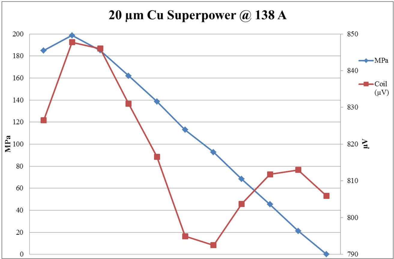
**Figure 49:** 20μm Coil compression behavior at 138 A
