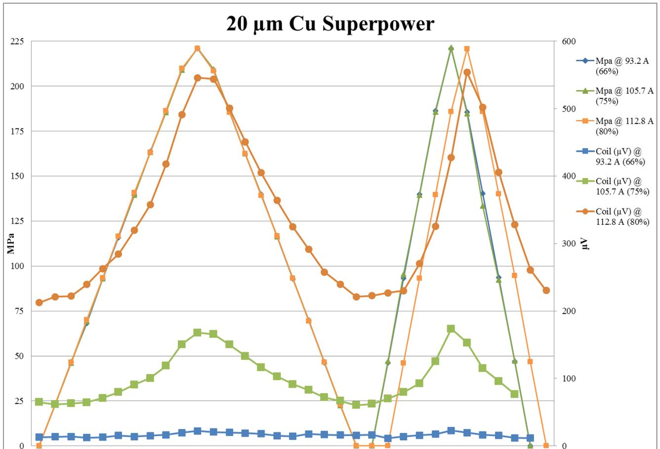
**Figure 60:** 20 $\mu$ m Coil compression behavior at 66%, 75%, and 80% original coil  $I_c$
