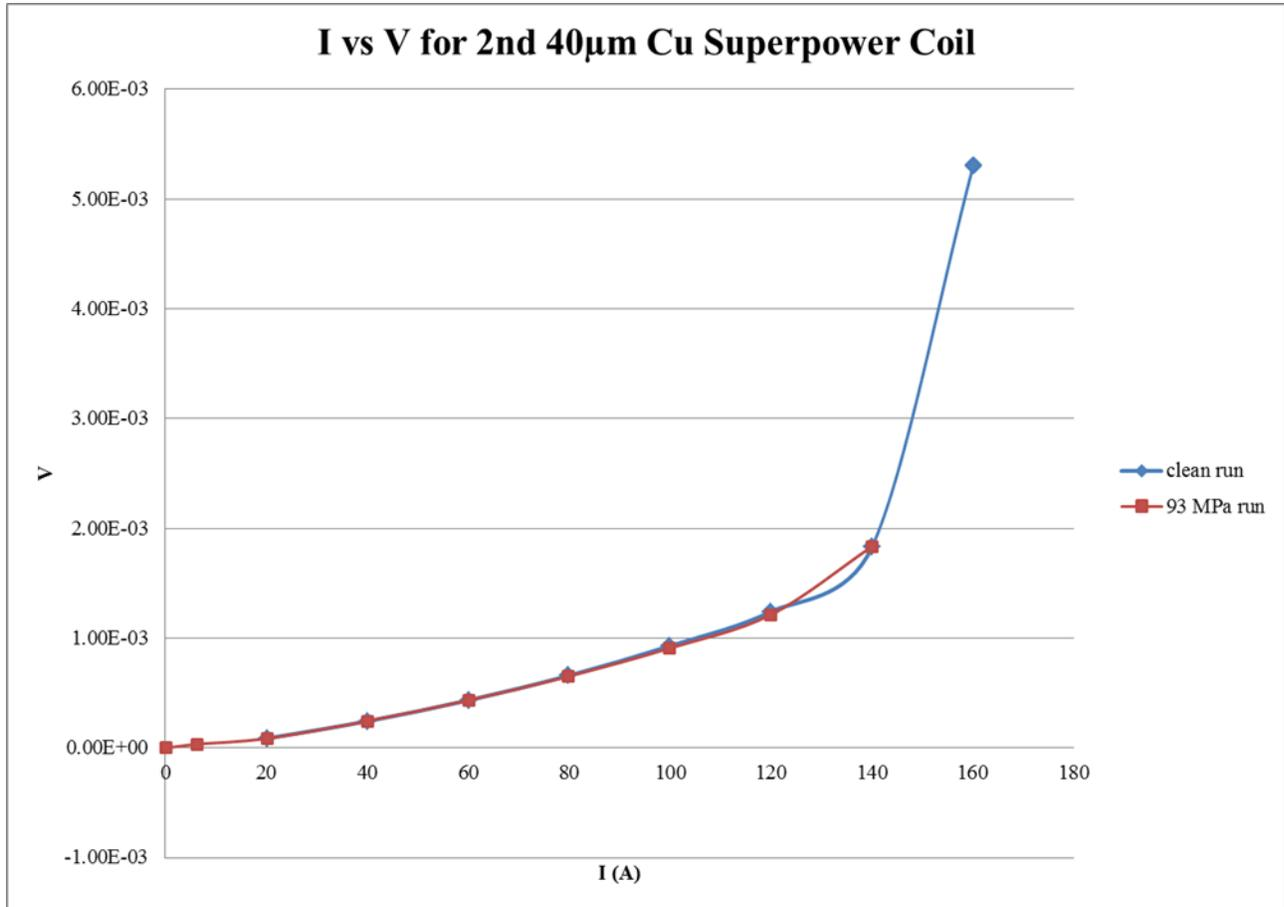
**Figure 21:** Initial I vs V for 2nd 40 $\mu\text{m}$  Coil
