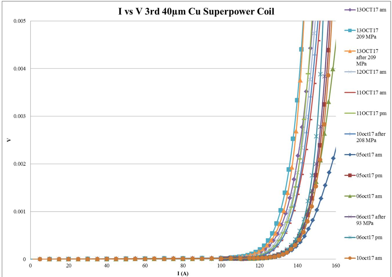
**Figure 30:** I vs V for 3rd 40 $\mu\text{m}$  Coil throughout its test time
