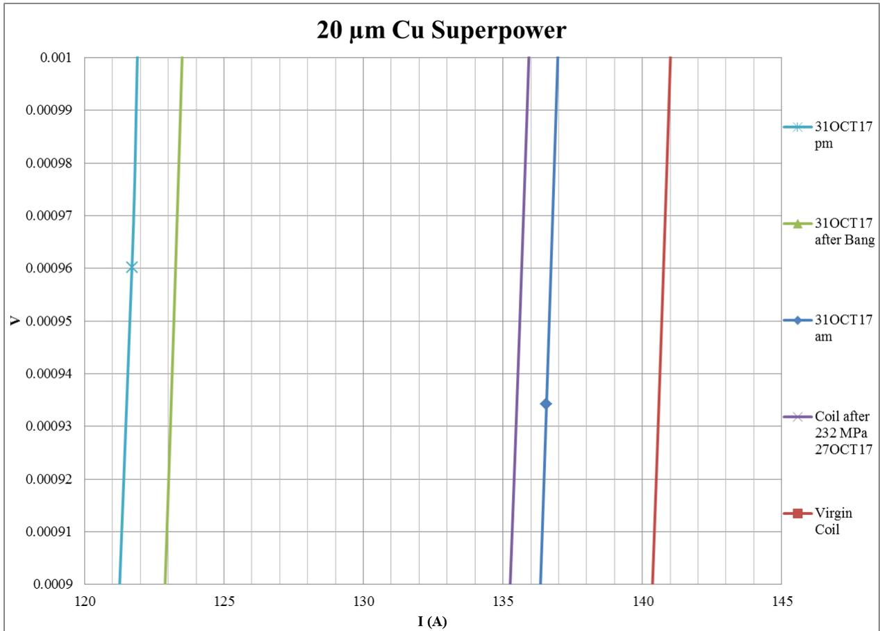
**Figure 62:** *I vs V for 20μm Coil*
