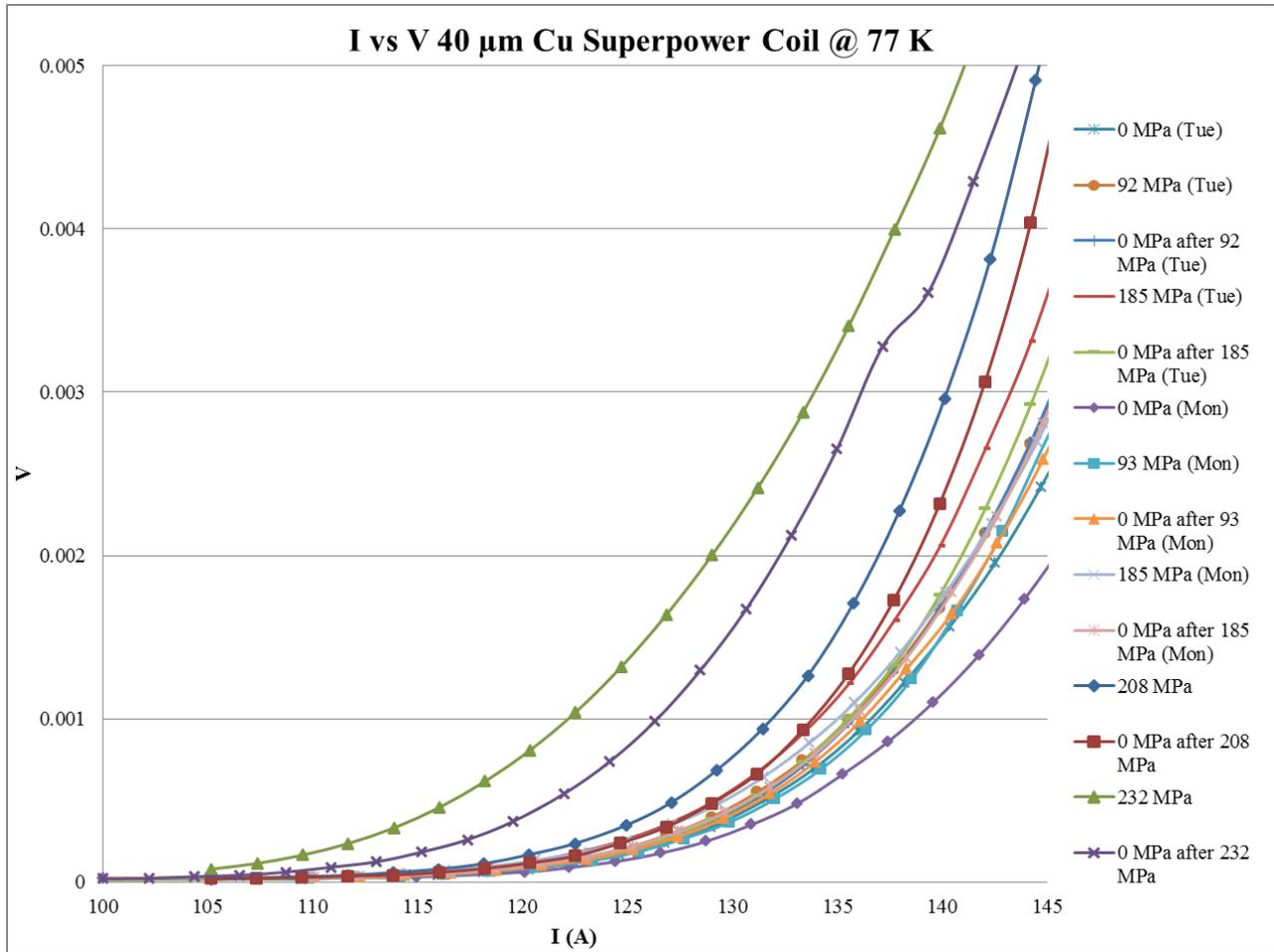
**Figure 25:** *I vs V for 2nd 40μm Coil @ 77K*
