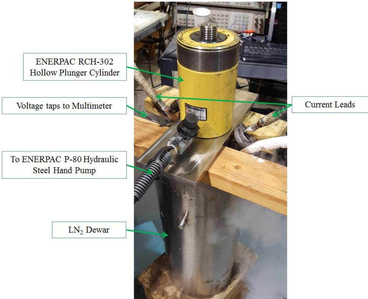
*Figure 5: Compression Test setup*
