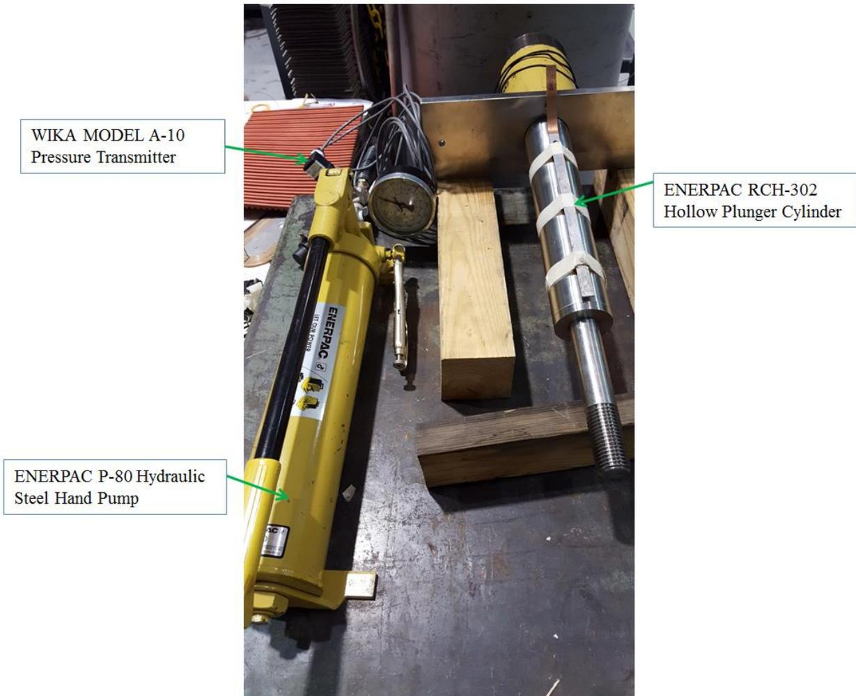
**Figure 4:** *Compressions fixture setup*
