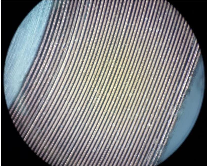
*Picture 3: Top of the coil after 100 MPa of compressive loading under a microscope*
