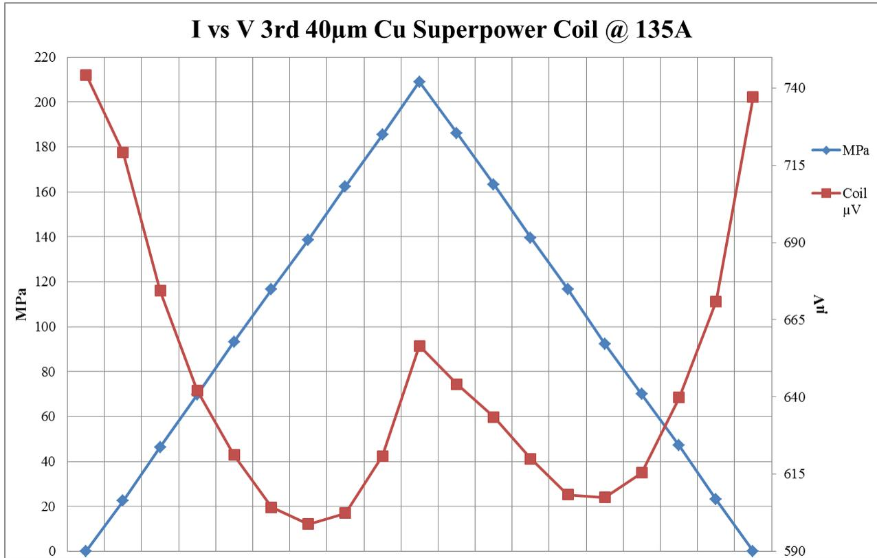
Figure 34: 3rd 40µm Coil compression behavior at 135 A
