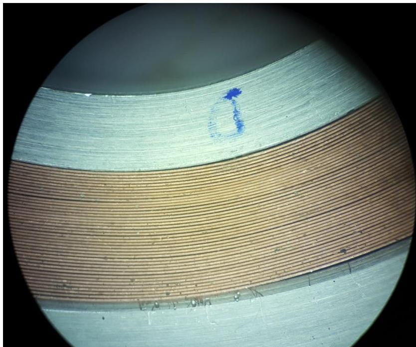
*Picture 6: Bottom of the coil after 175 MPa of compressive loading under a microscope*
