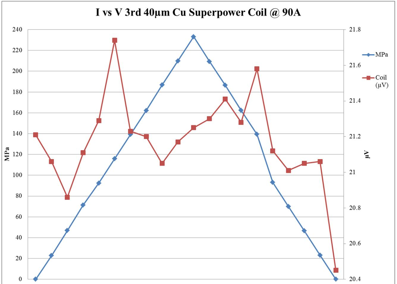
**Figure 40:** 3rd 40µm Coil compression behavior at 90 A
