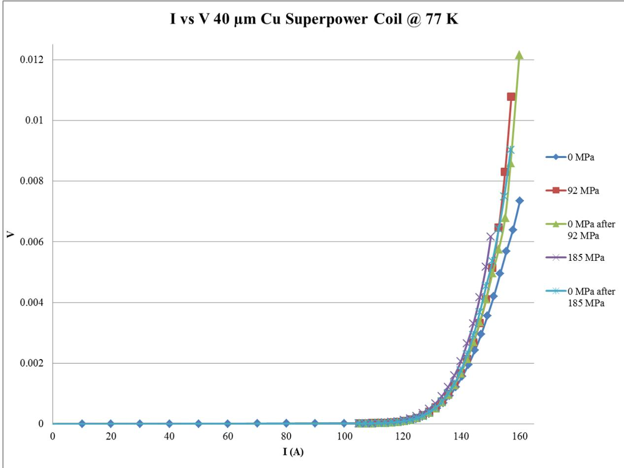
Figure 22: I vs V for 2nd 40μm Coil @ 77K
