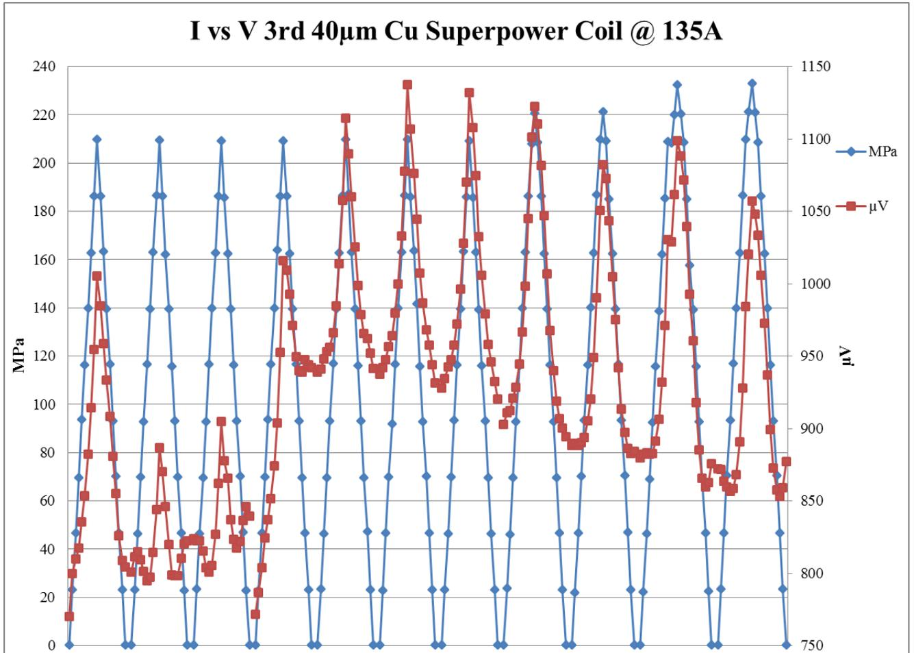
Figure 36: 3rd 40µm Coil compression behavior at 135 A
