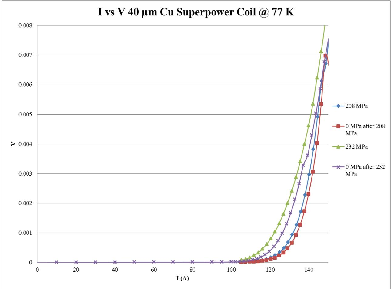
**Figure 26:** I vs V for 2nd 40μm Coil with and without compressive pressure
