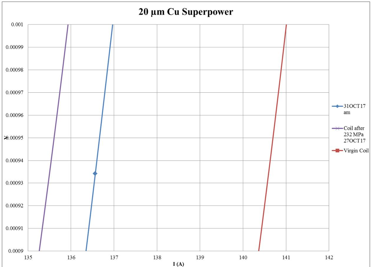
Figure 55: I vs V for 20μm Coil
