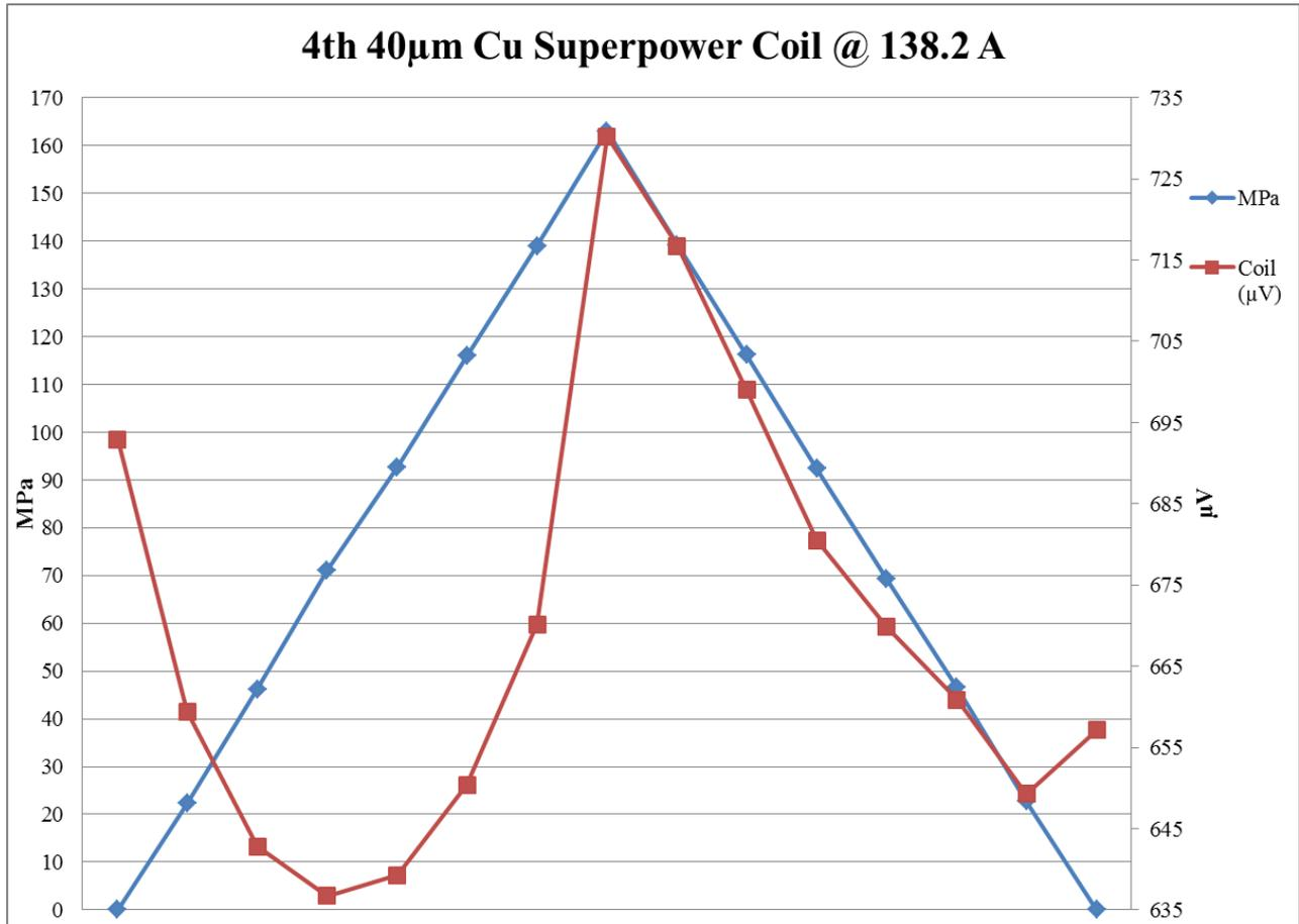
**Figure 45:** 4th 40µm Coil compression behavior at 138.2 A
