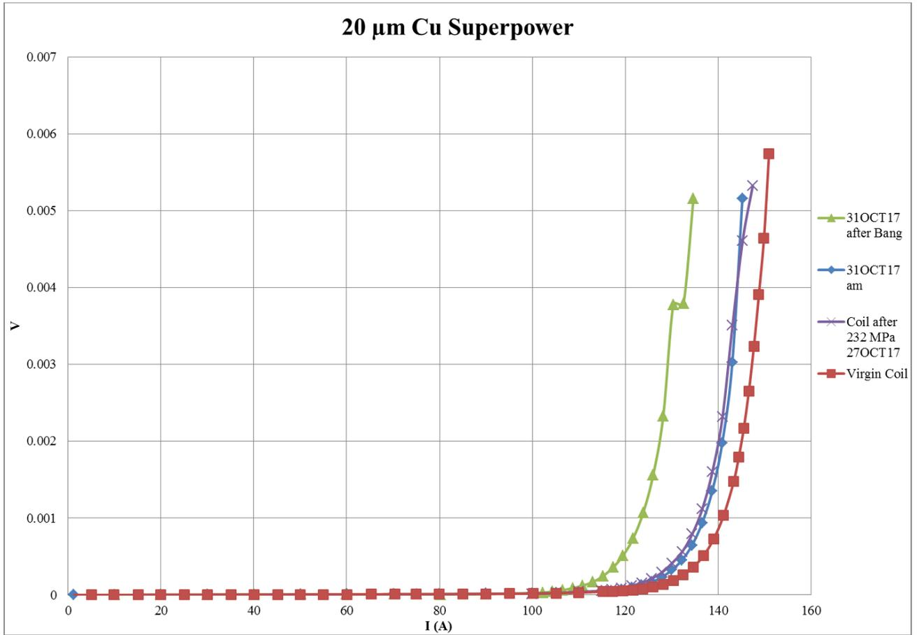
Figure 58: I vs V for 20μm Coil
