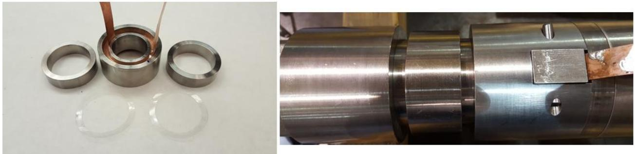
**Figure 12:** *Stainless Steel outer ring and double piston – optimal design; added 5 mil Mylar caps to top and bottom of coil for even compression force distribution and to prevent bypass current*
