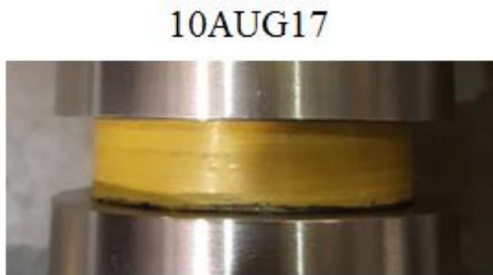
*Figure 6: Kevlar wrapping reinforced by Epoxy – inefficient to remove and replace after every inspection and time consuming to wrap and dry*
