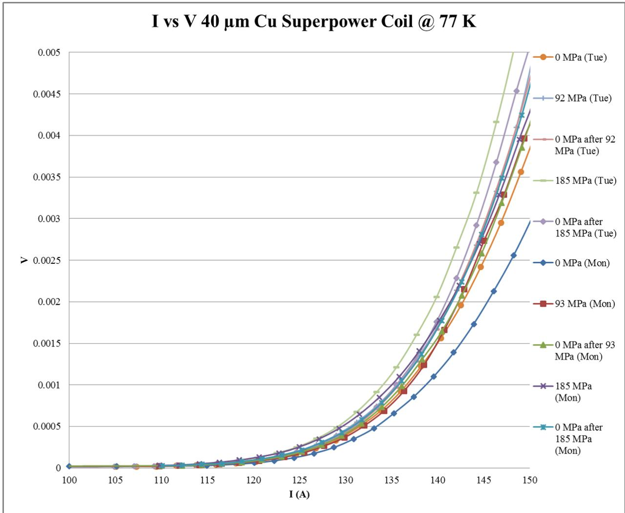
Figure 24: I vs V for 2nd 40μm Coil @ 77K
