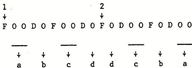
where a single 0 represents a short drift (S) and two 0's, a long drift (L), and where 1 and 2 are the two reflection symmetry points. The magnets are shifted symmetrically away from 1 and towards 2, thus modulating both the bending and the focusing properties of the lattice.
