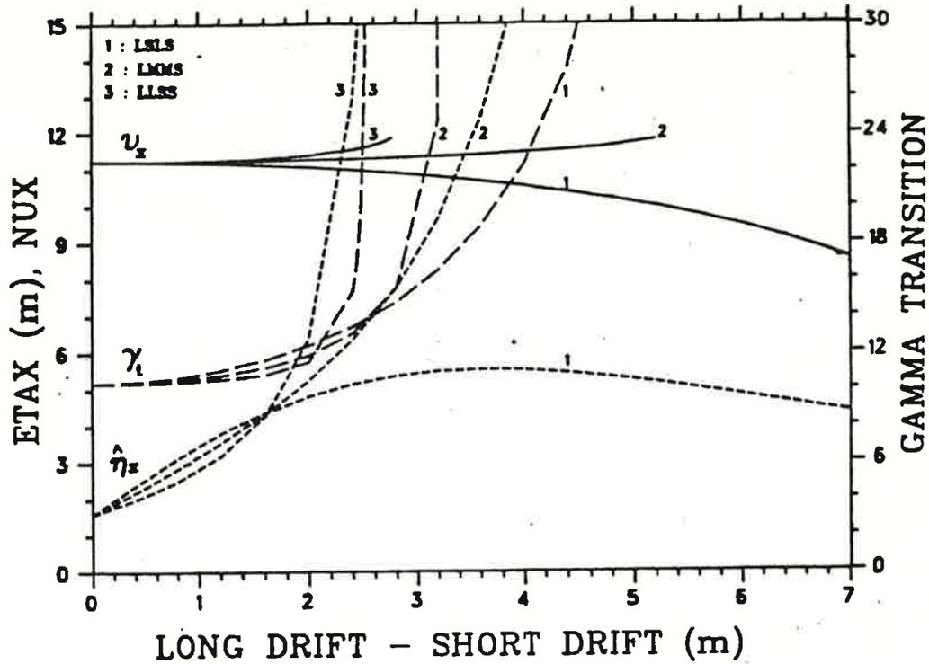
Fig. 5. Effects of increasing the difference between the long and the short drifts starting from a regular lattice. Patterns examined: 1:LSLS, 2:LMMS and 3:LLSS ( $M = 3.5$  m = drift length in a regular lattice). In this figure  $v_x$ ,  $\hat{\eta}_x$  and  $\gamma_t$  are shown (Ref. Ch. 4).
