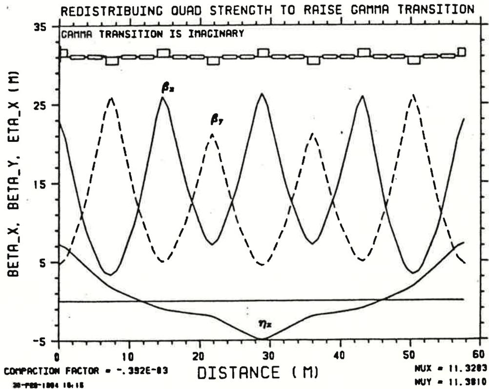
Fig. 2. Raising transition energy by modulating the quadrupole lengths. The length of the quadrupoles at the two symmetry points are respectively 1.98 m and 1.45. The compaction factor has become negative and  $\gamma_t$  imaginary. Length of all quads in a regular lattice will be 1.7 m. (Ref. Sec. 3.2).
