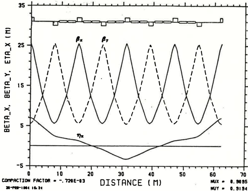
Fig. 3. Raising transition energy using missing magnet cells. In this example one of the four cells is empty.  $v_x/n$  is .9095 and  $n$ , the no. of superperiods, is 12. (Ref. Sec. 3.3 (a)).
