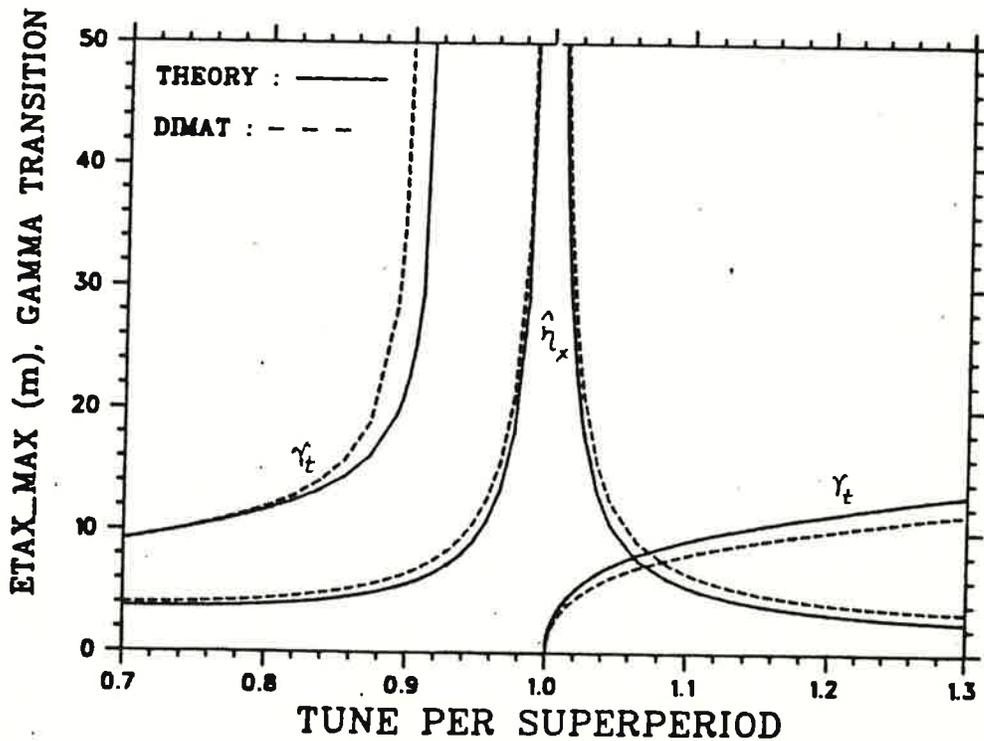
Fig. 4. Comparison of the dispersion and  $\gamma_t$  for the computed results using the formulas derived in Sec. 3.3 (a) and the results obtained from the lattice code DIMAT in the missing magnet cells method. (Ref. Sec. 3.3 (a)).
