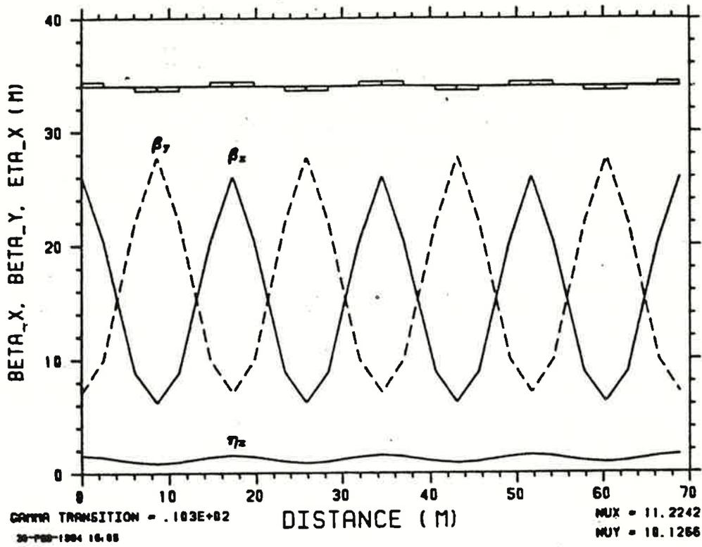
Fig. 1. Regular lattice consisting of CERN/ISR magnets. The transition energy is in the range of acceleration. (Ref. Ch. 1).
