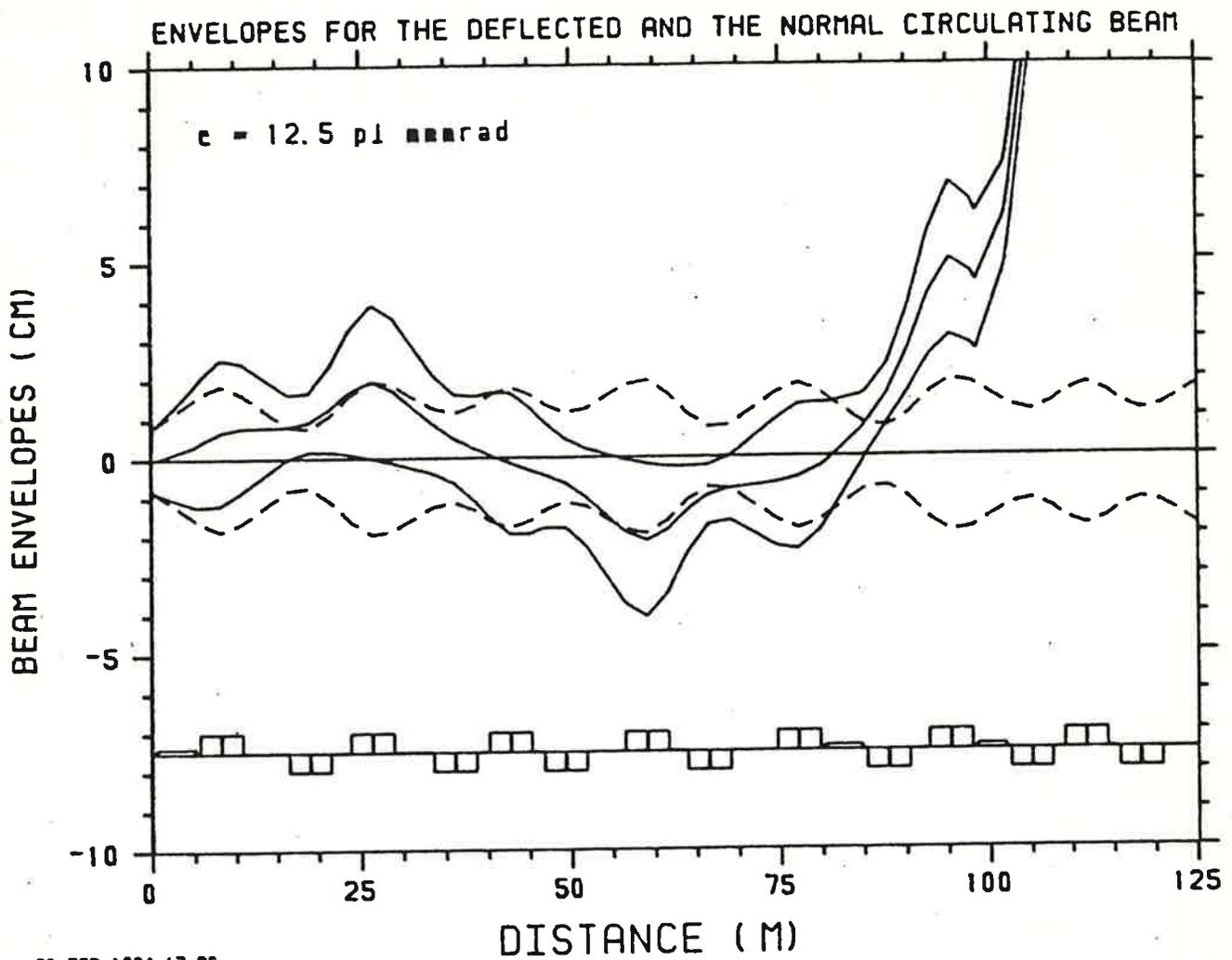
Fig. 11. A fast extraction system for the main synchrotron. Long drifts of the unequal drift lattice of Fig. 10 have been utilized for placing the two kickers and one septum magnet. (Ref. Appendix A).
