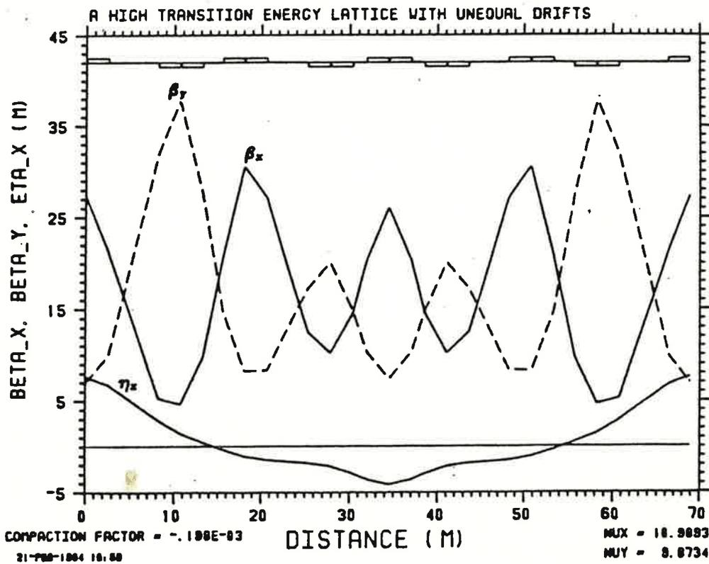
Fig. 10. A lattice optimized for high transition energy and low peak values of the lattice functions. A complete parameter list is given in Table 2. (Ref. Ch. 4).
