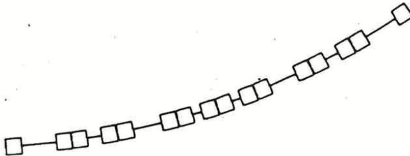
Fig. 9. Layout of one superperiod. A relatively higher magnet density is created at the mid-point. This provides the desired harmonic to increase  $\gamma_z$ , (see lattice below). There are 12 superperiods in the main synchrotron. (Ref. Ch. 4).
