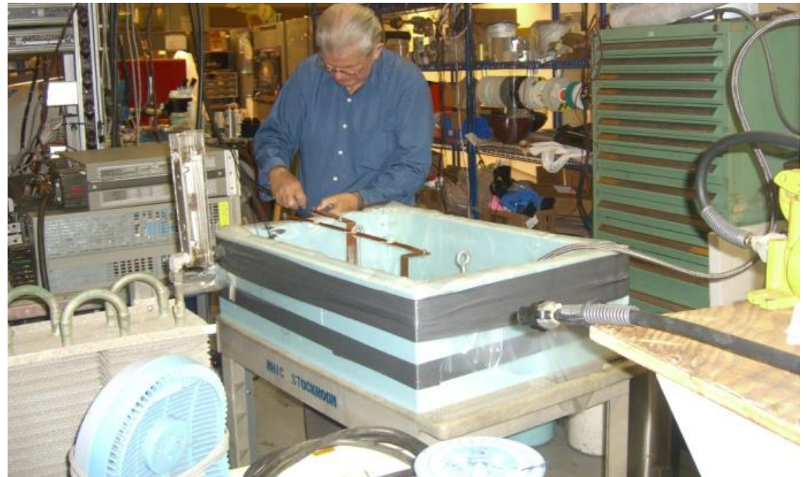
Cryostat made with Styrofoam and Duct-tape
