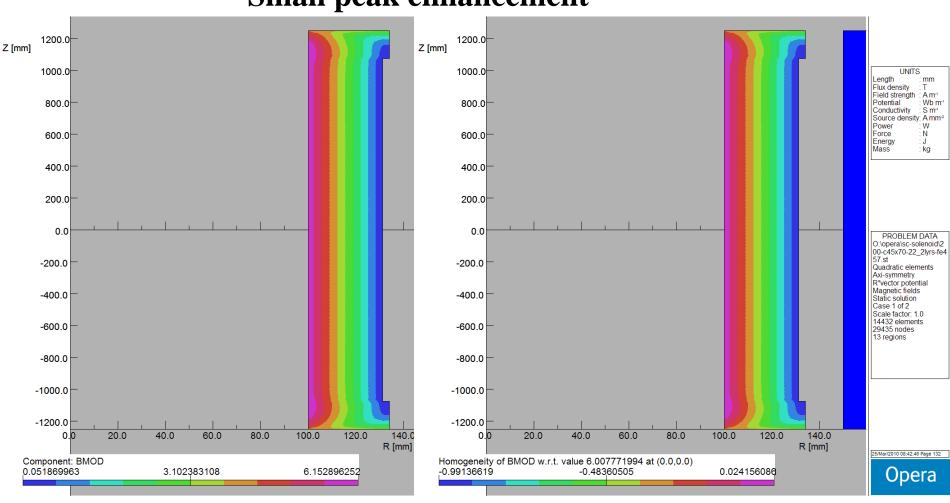
only 2.4% enhancement of field on the conductor
