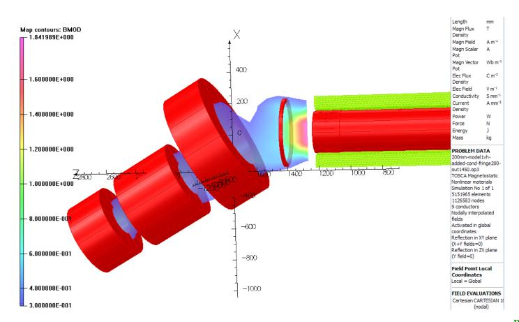
A more efficient location of fringe field coil may be a bit off-axis.
