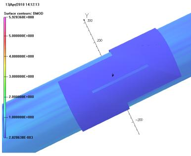
Desired Field is obtained at 13.8 A (~50% more than optimum integral)
