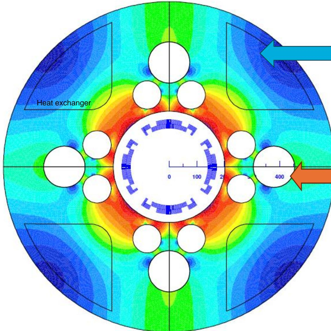
Remove iron from the areas where it is not saturated (includes heat exchanger)
