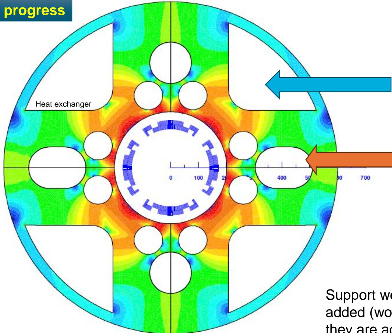
Iron removed to make yoke lighter
