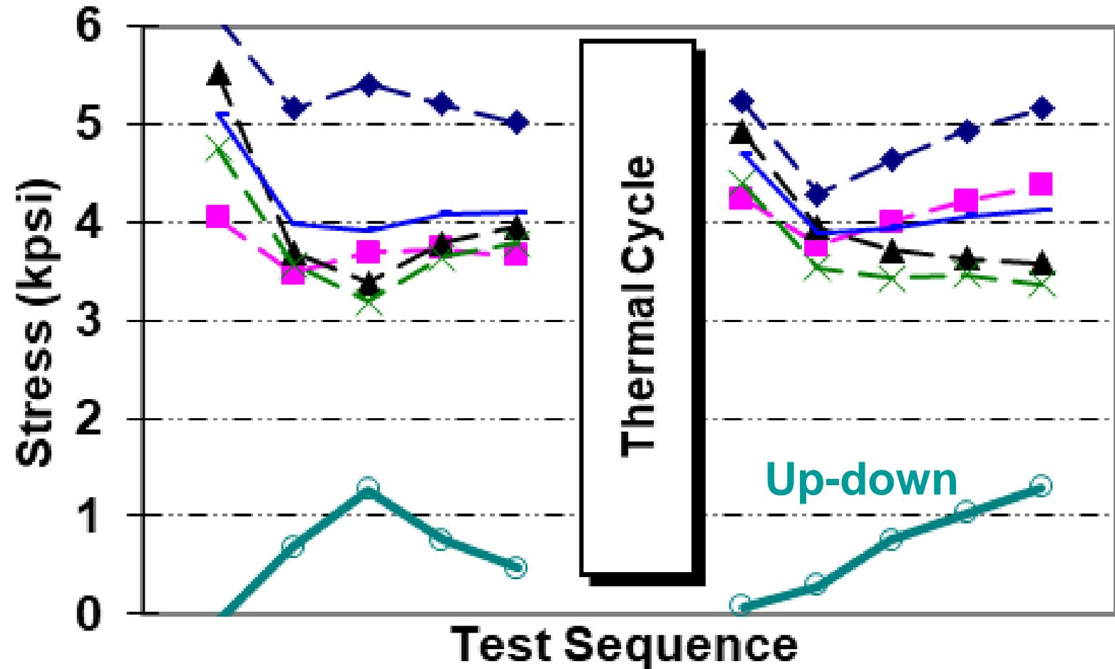
The azimuthal stress on pole faces (dashed lines), average (solid) and difference between top and bottom (thick solid line) after successive quenches together with a thermal cycle in between in the magnet DRZ105.
