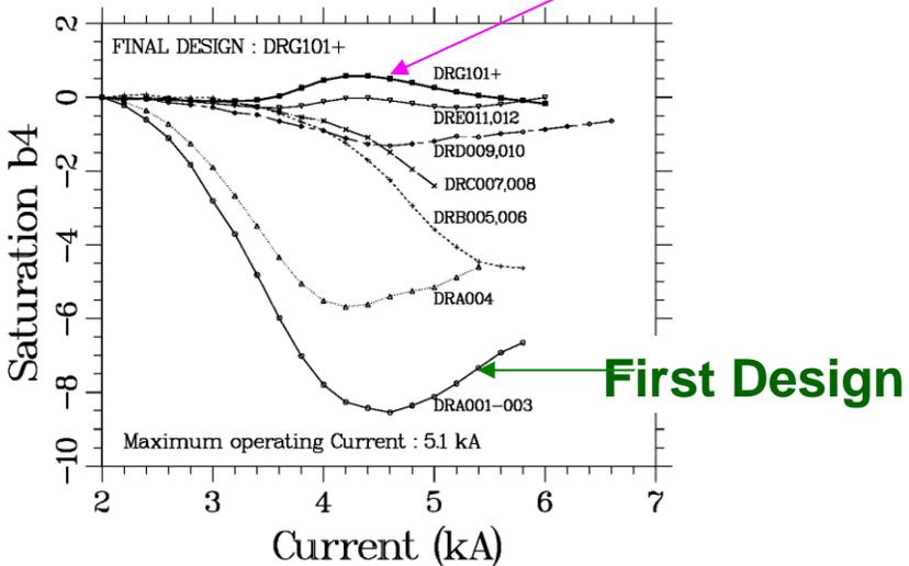
Current Dependence in RHIC Dipole DRG107 (DC Loop, Up Ramp)
