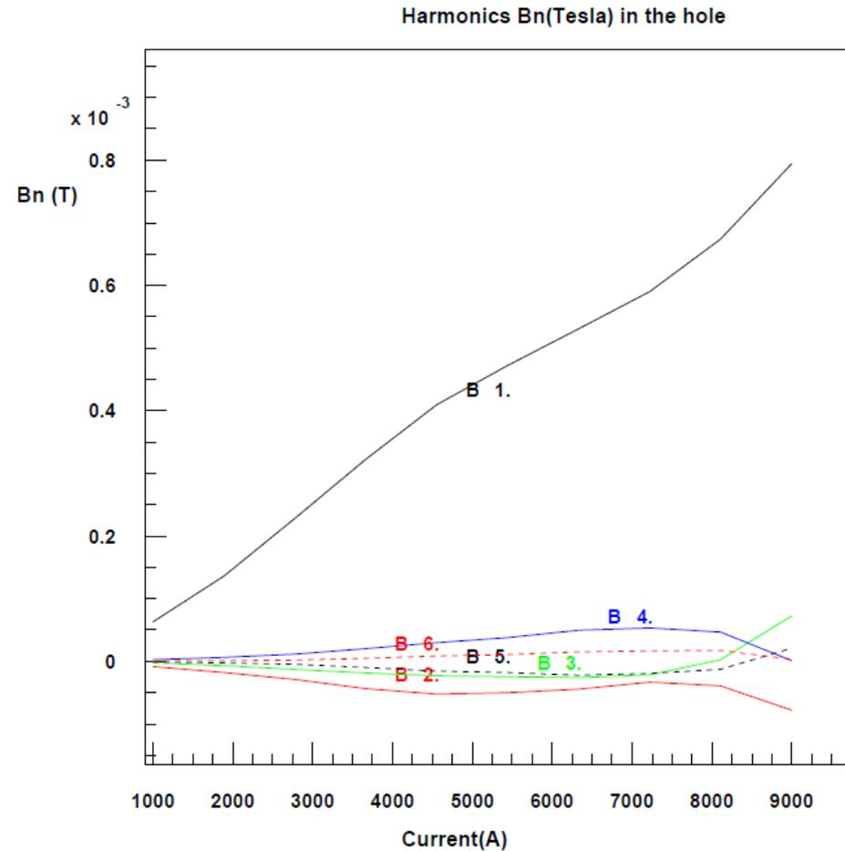
**Harmonics  $B_n$  in Tesla remain  $<10^{-4}$  units at 50 mm radius.**
