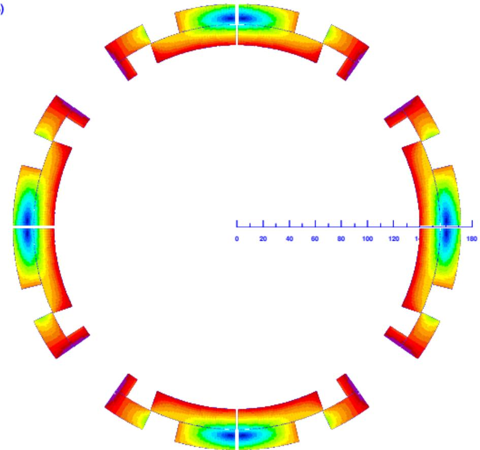
Design optimized to reduce peak field enhancement (max field on the cable over the field at midplane) to ~18%
