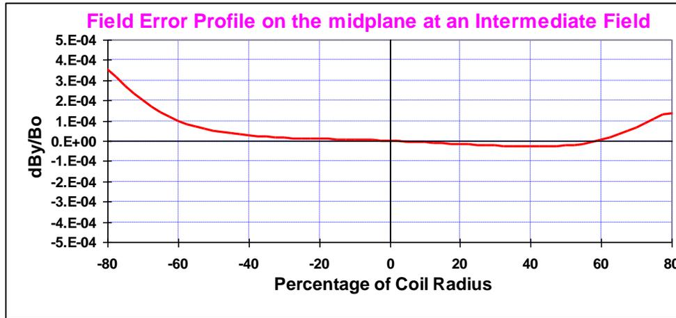
Field errors within  $10^{-4}$  at 60% of coil radius, and  $\sim 4 \cdot 10^{-4}$  at 80% in the first magnet itself
