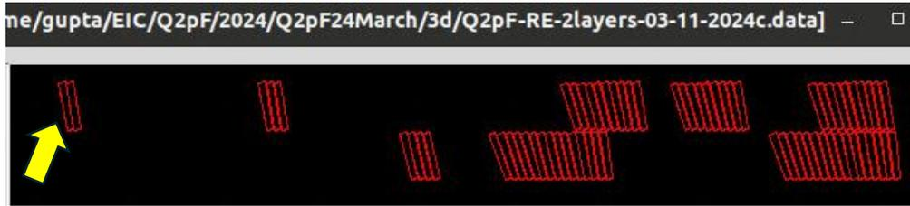
End configuration iterated for smaller peak fields in the ends.
