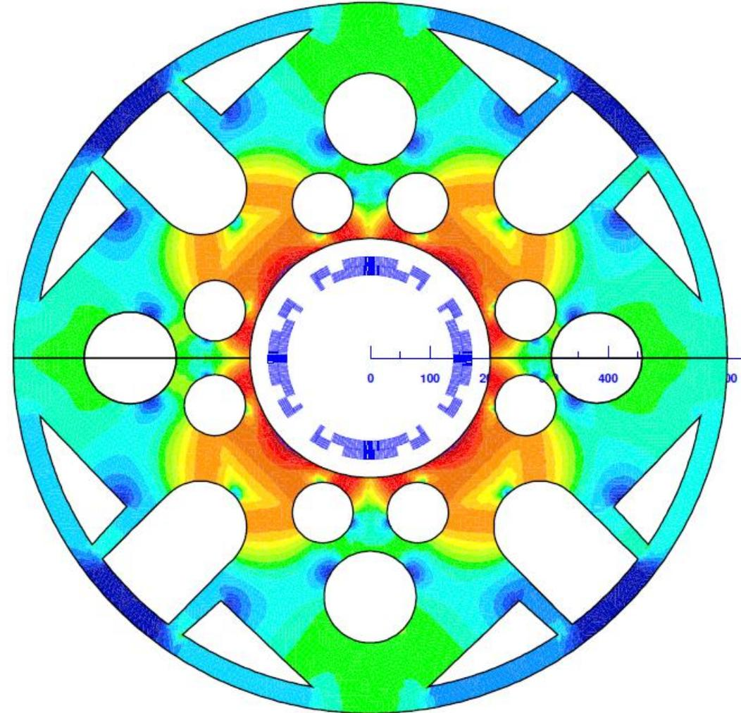
Iron removed to make yoke lighter
