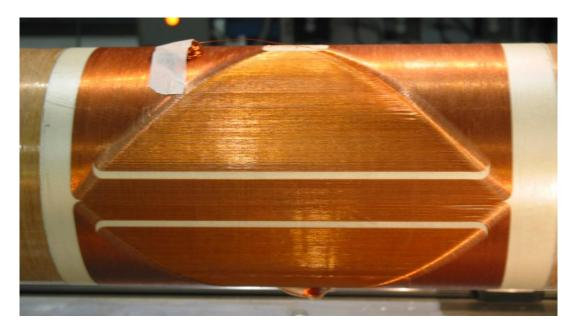
Turns at midplane contribute much more to field than turns at any other angle. In the "Optimum Integral Design" midplane turns extend full-length
