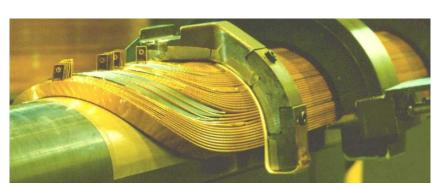
Fewer coils (about half) as the same coils are common between the two apertures (2-in-1 geometry for both iron and coils)
