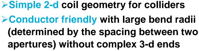
Facilitates many conductors (High current HTS cables) and technologies (React & Wind)
