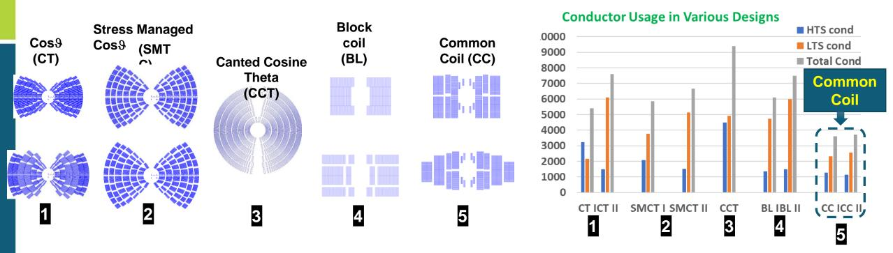
Comparative studies of 20 T designs (as presented at MT) revealed that the common coil design uses significantly less conductor than the other designs.
