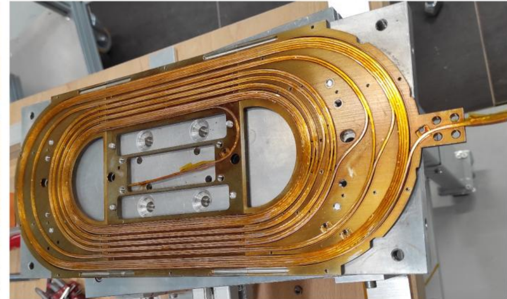
View of the coil before the soldering process
