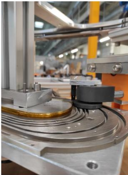
Winding: the insulated cable is assembled during the winding process
