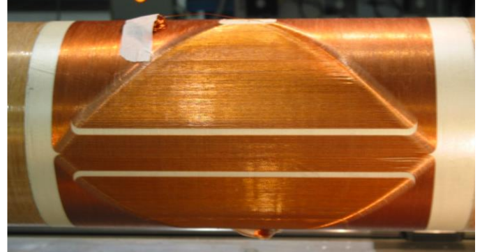
Fig. 4. An AGS corrector dipole coil built based on the Optimum Integral Design . One can note that the midplane turns span almost the full end-to-end coil length and the coil has a high fill factor of superconducting wires.
