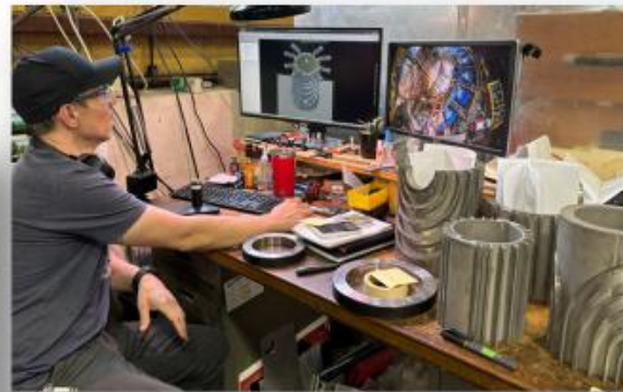
3D printed 316L coil mandrel, QC and postprocessing
