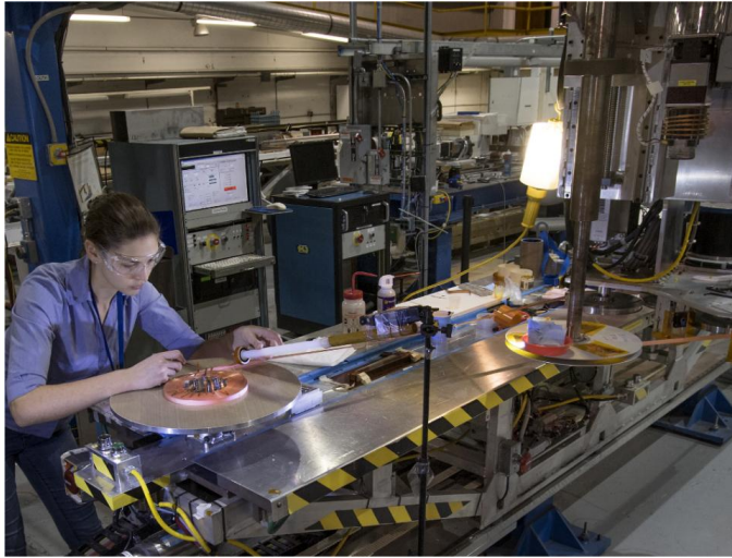
No-insulation coil winding for IBS (id 105 mm, od=200 mm)
