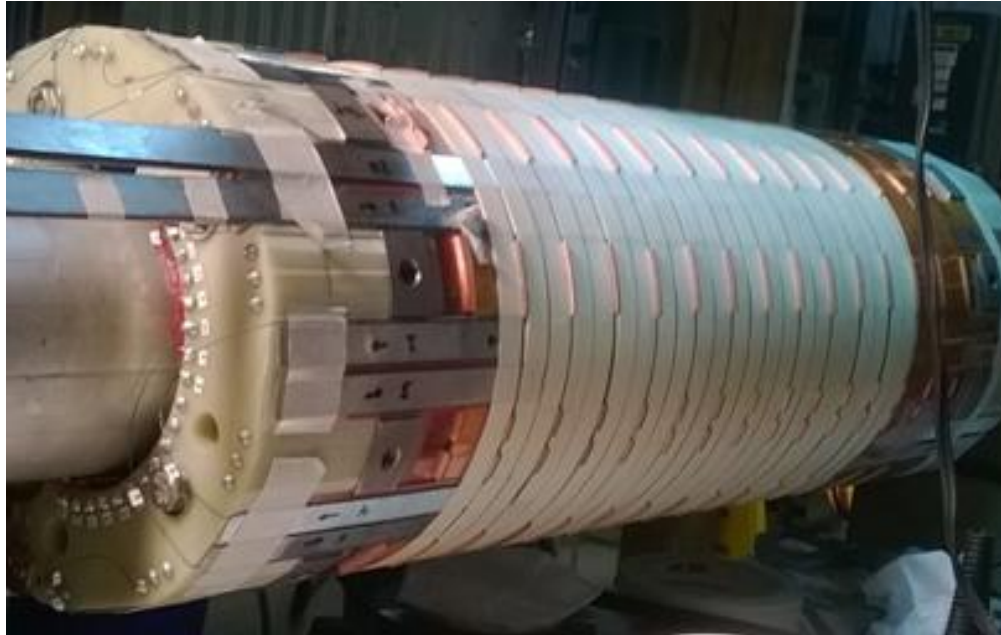
Inner Solenoidal Coil (102 mm id, 194 mm od) 28 pancakes
