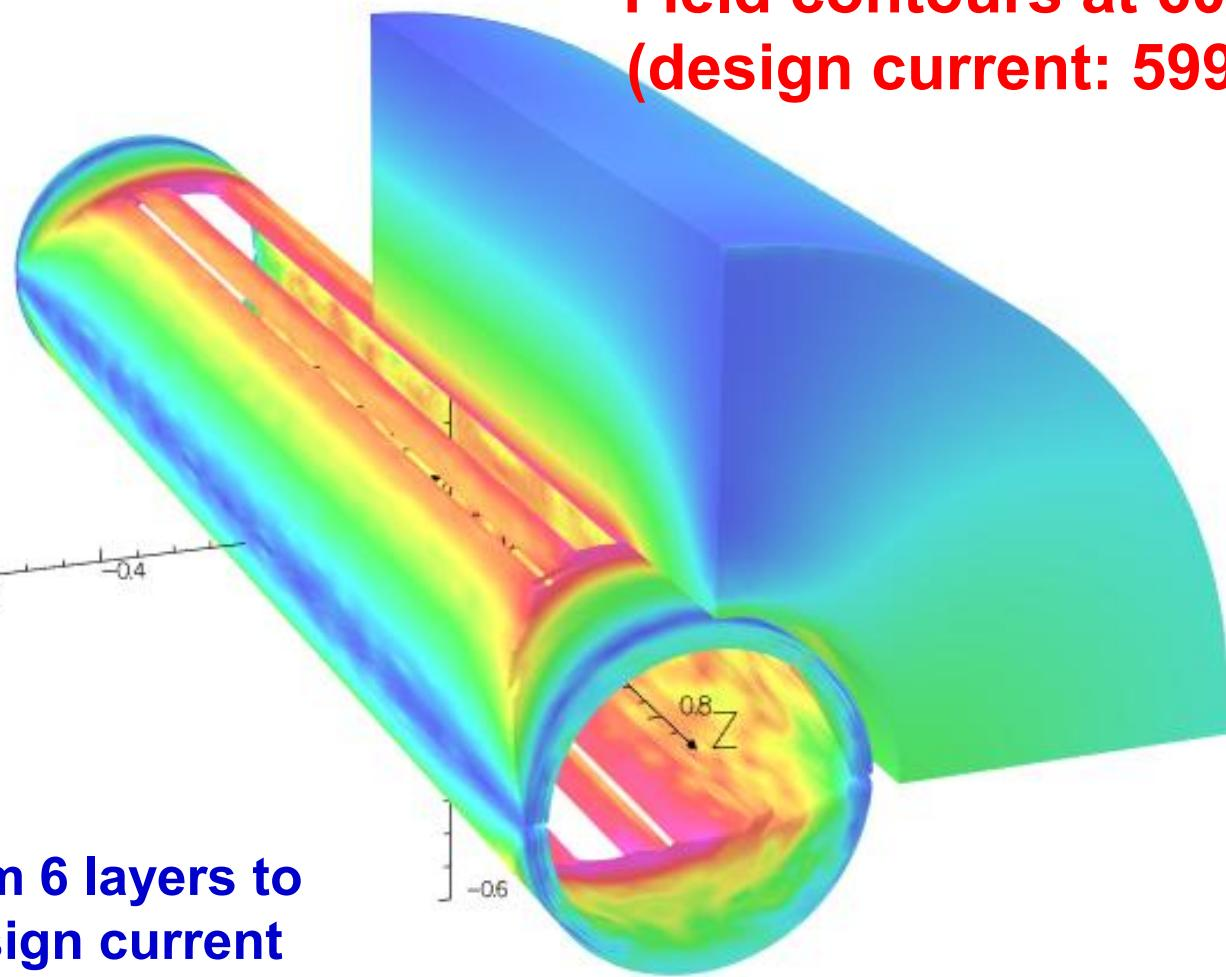
In going from 6 layers to 8 layers, design current reduced from 786 A to 599 A
