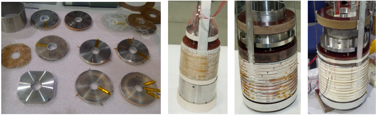
Fig. 1a-d.: High field HTS solenoids designed, built and tested by PBL/BNL collaborations. Left: 25-mm bore pancake coils for insert magnet. Left-center: Solenoid that generated 16 T. Right-center: Solenoid with 12 double-pancakes of 100 mm bore. Right: Nested set.
