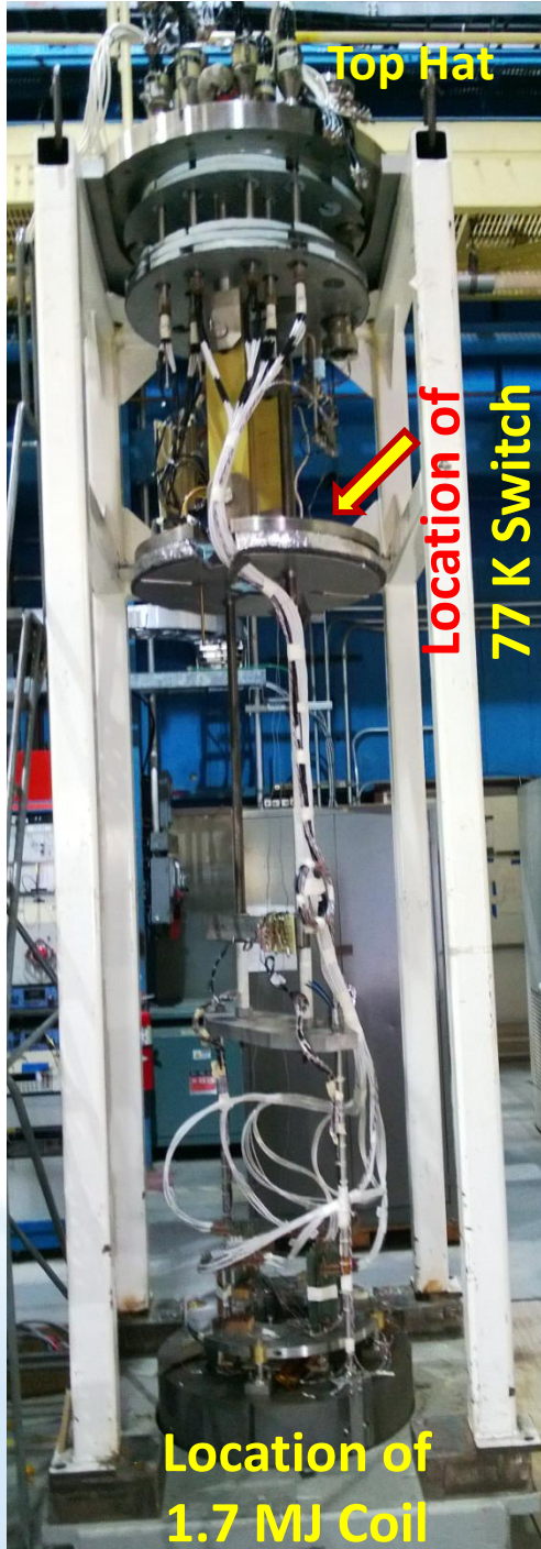
Top Hat with instrumentation panel and current leads
