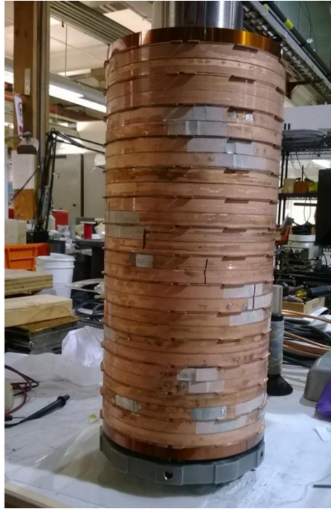
Fig. 3: Inner coil consisting of all (28) HTS pancakes assembled on the inner tube.
