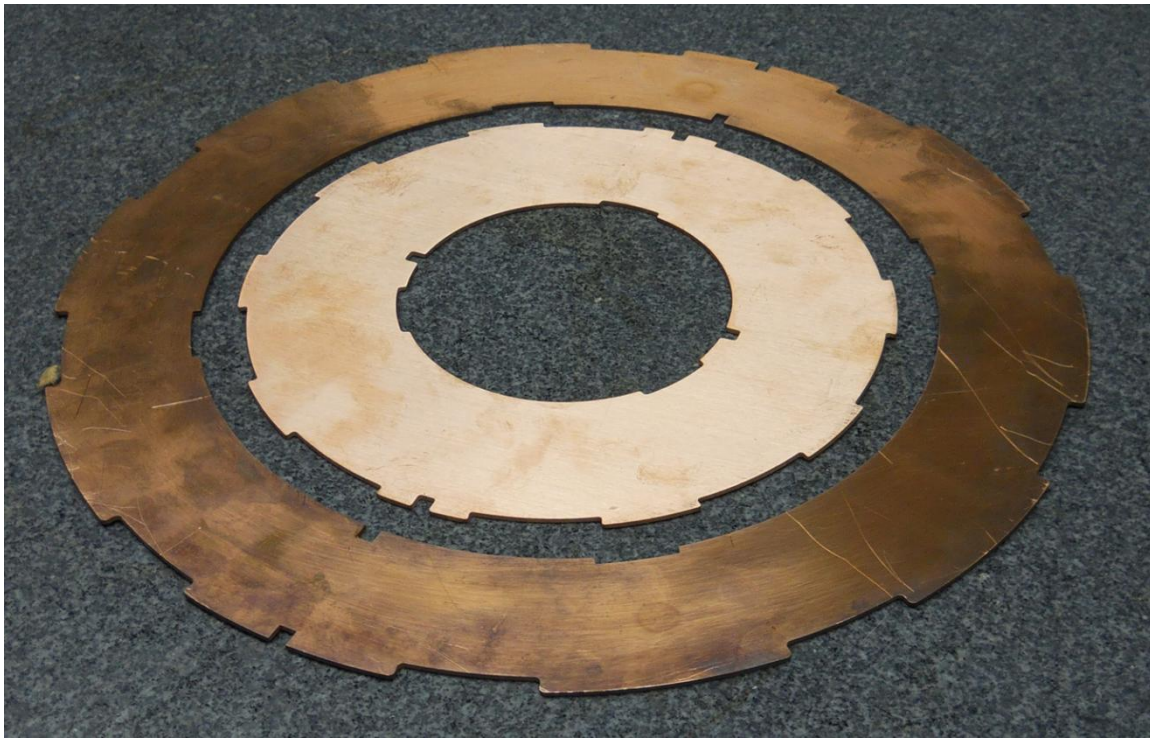
Fig. 2: Copper disks for inner and outer coils. These copper disks will be placed on either side of each double pancake during the final assembly.
