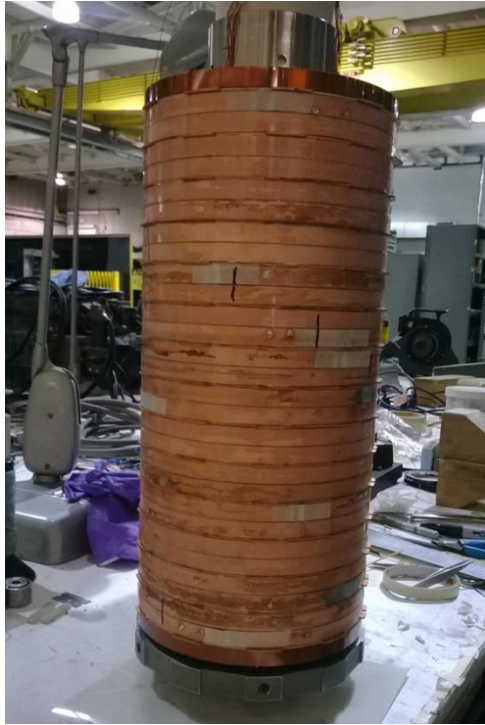
Fig. 3: Inner coil consisting of all (28) HTS pancakes assembled on the inner tube.
