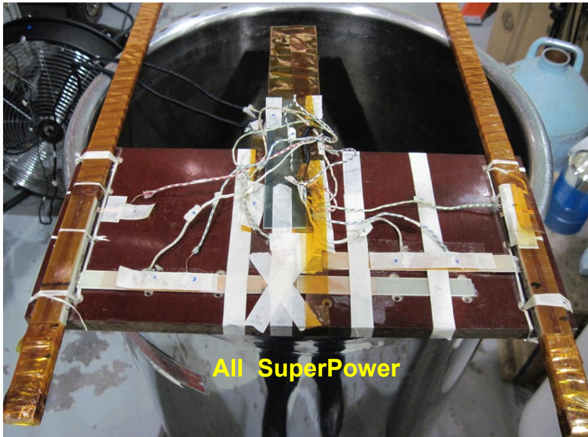
Fig. 3: Development and test of lead joint for outer coil.
