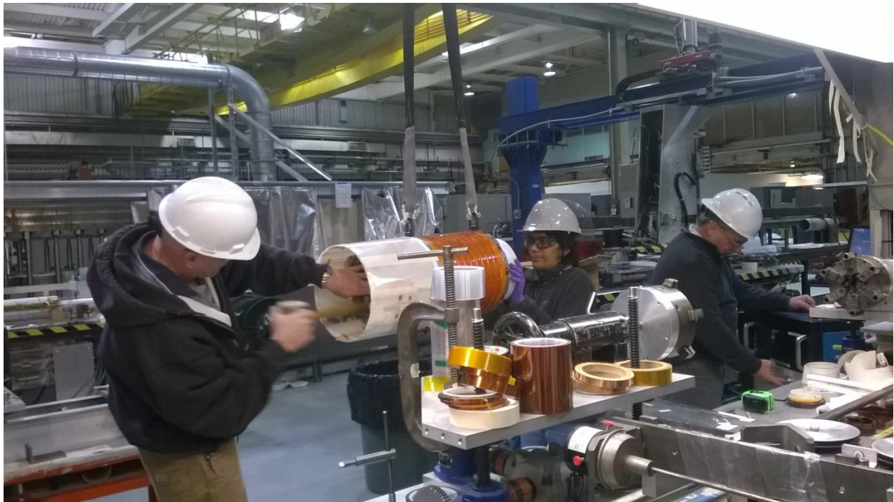
Figure 13: Preparation is being made to put Kevlar string over the outer layer.
