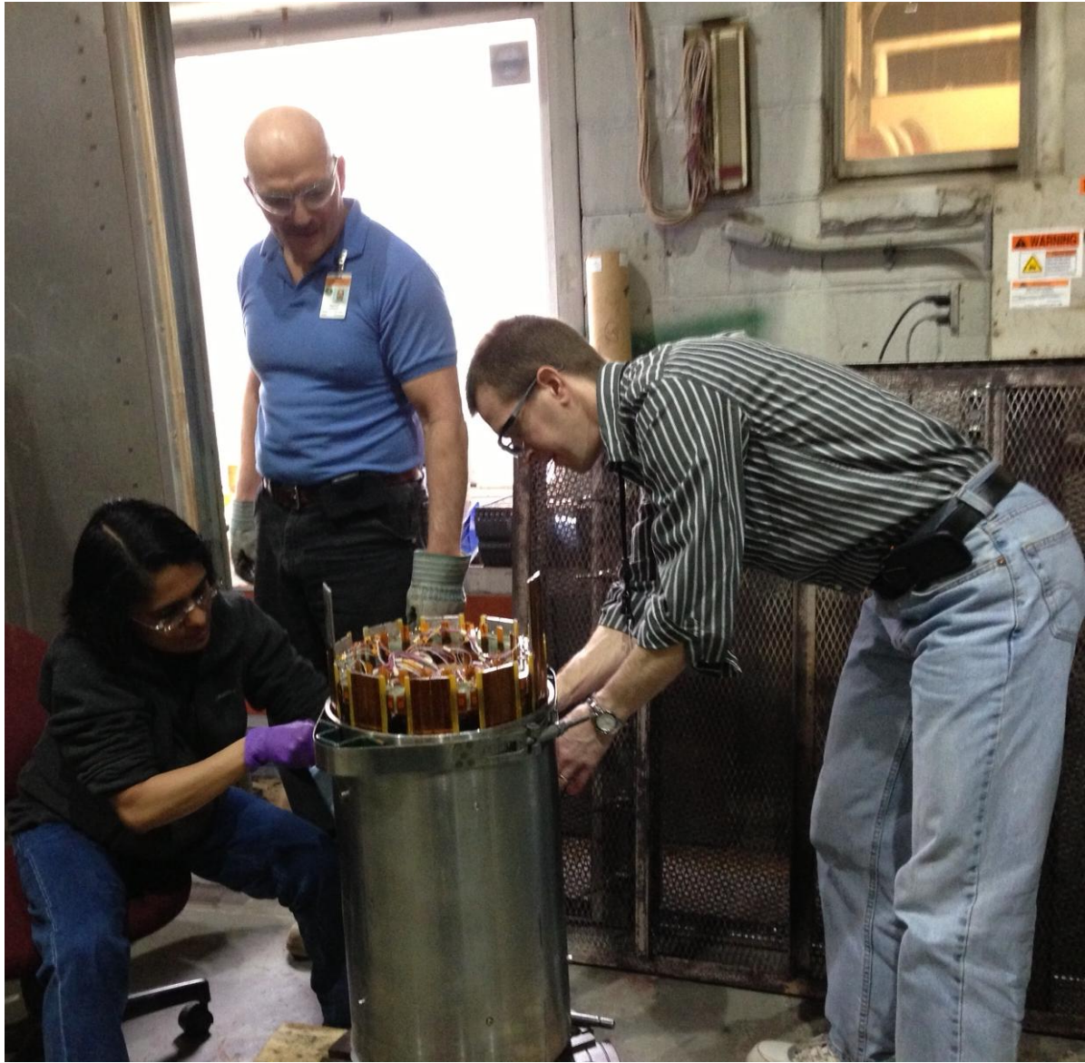
Figure 19: Outer coil with stainless steel support tube installed.
