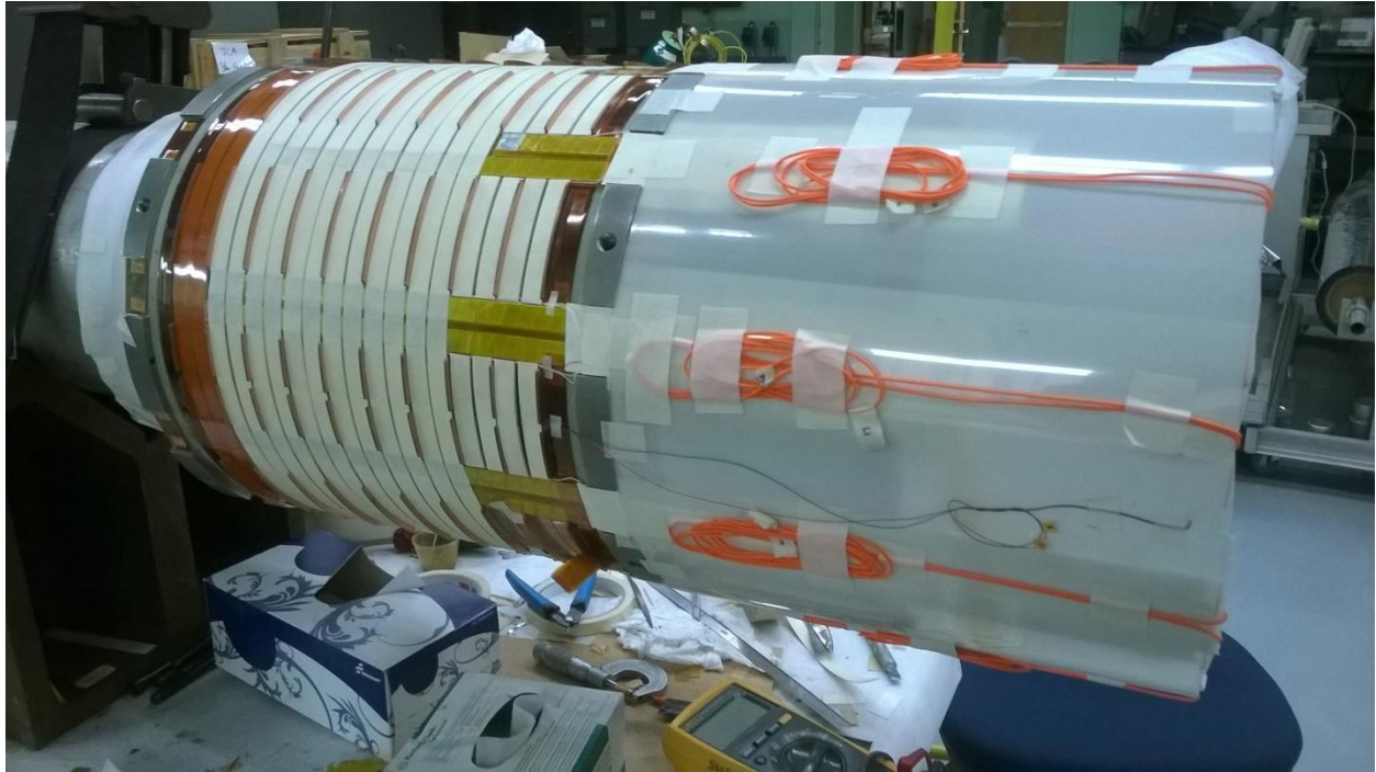
Figure 12: Nomex filler pieces placed in between all leads and around several pancakes of outer layer.
