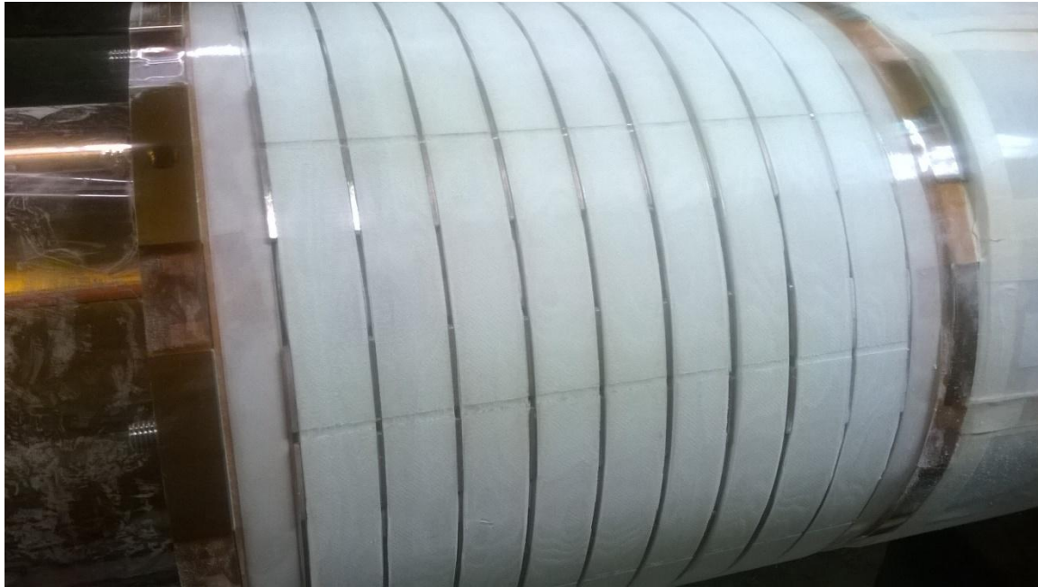
Figure 16: Outer pancake after outer diameter machined to the required dimensions and axial grooves for helium cut.
