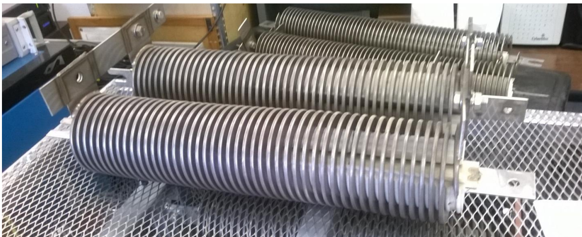
Figure 23: Part of the external dump resistor system for extracting 1.7 MJ of energy.
