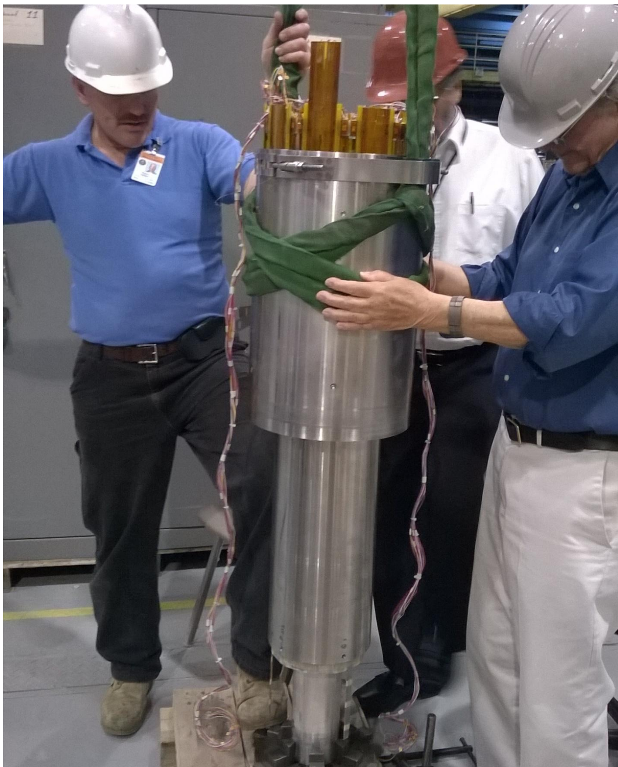
Figure 20: Outer coil with support structure being inserted over the inner coil with support structure.
