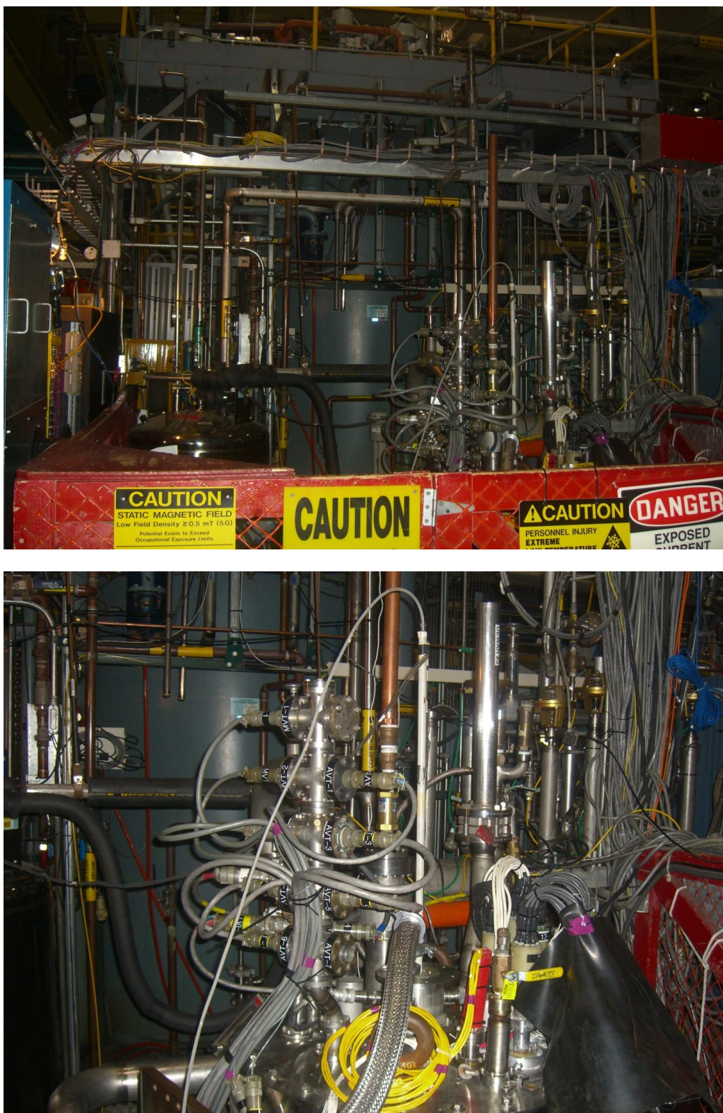
Figure 24: Instrumentation package used during the test of the HTS FRIB quadrupole. A similar package will be used for SMES.
