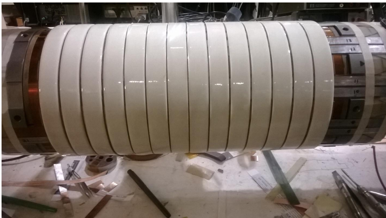
Figure 4: Completely cured inner pancake coil assembly.
