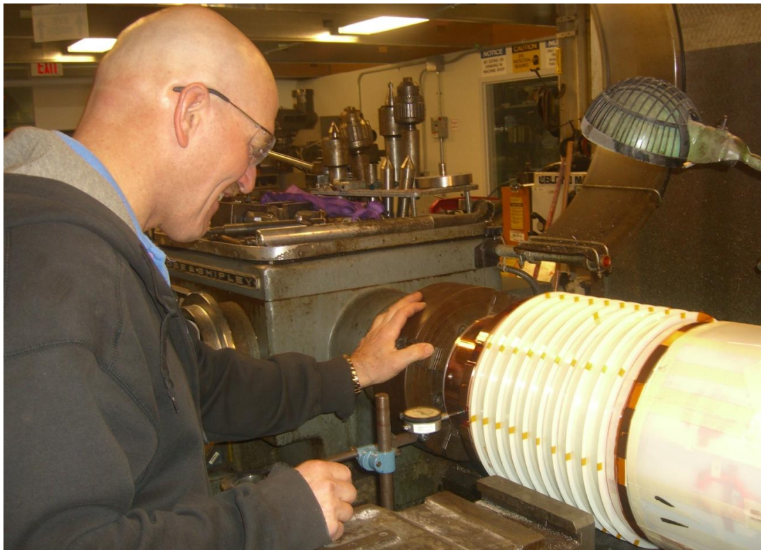
Figure 15: Outer pancake after curing. The coil is put on the fixture so that the outer diameter of it can be machined to required dimensions.
