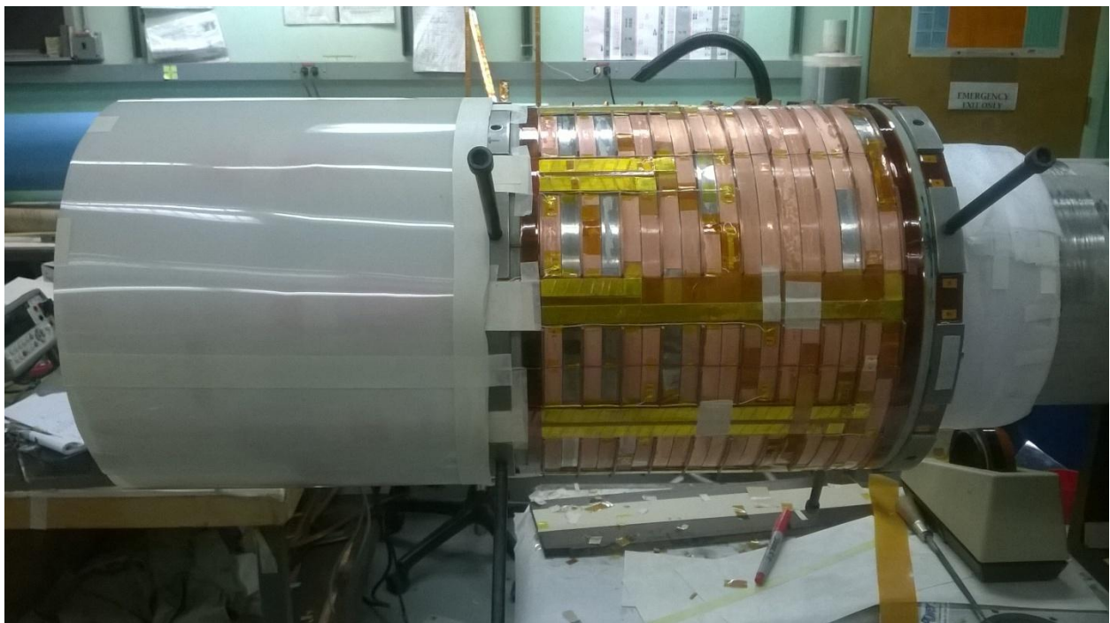
Figure 9: Leads installed (running across axially) for outer pancake coil assembly.
