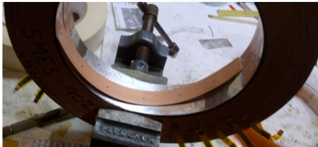
Internal splice in a double pancake coil
