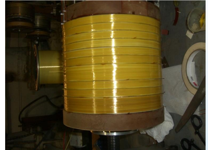
After wet-wrap of Kevlar and epoxy
