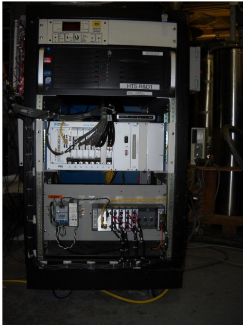
Fig. 7: Hardware (left) and screenshot of Labview software (right) for the quench protection system of SMES.
