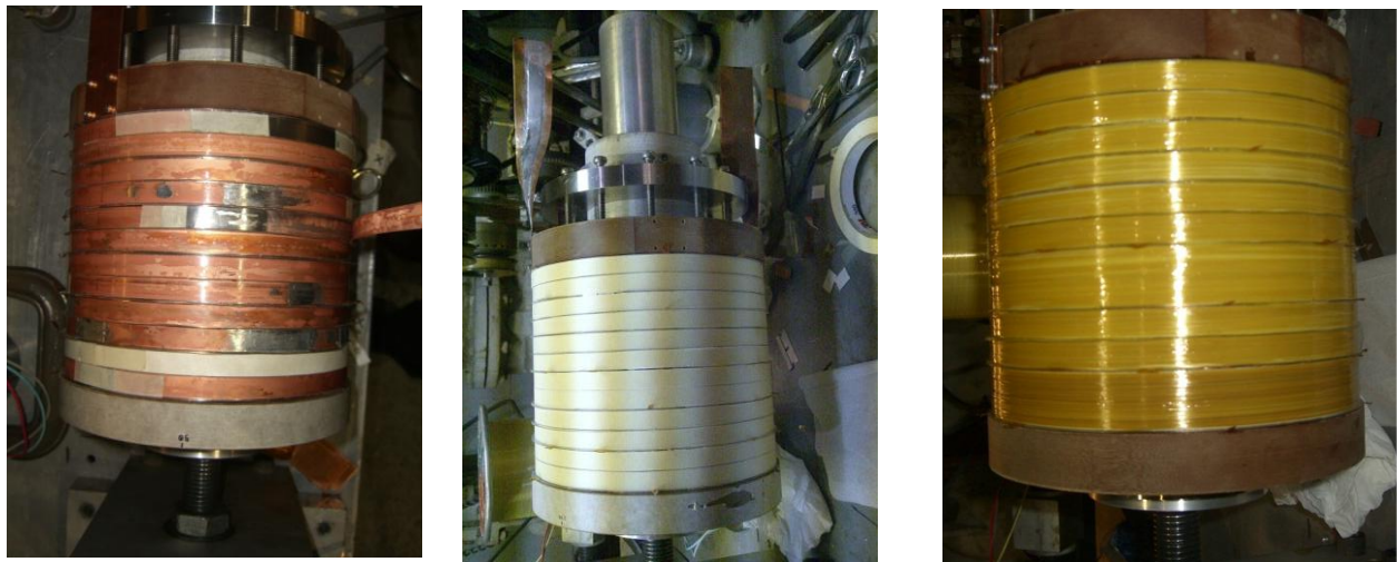
Fig. 9: Various steps of fabrication process of the SMES coil made to meet Go/NoGo milestone. Initial stack-up of 12 pancake coil is shown on the left, after all splicing and Nomex wrap in the middle and after wet-wrap of Kevlar and epoxy on the right.
