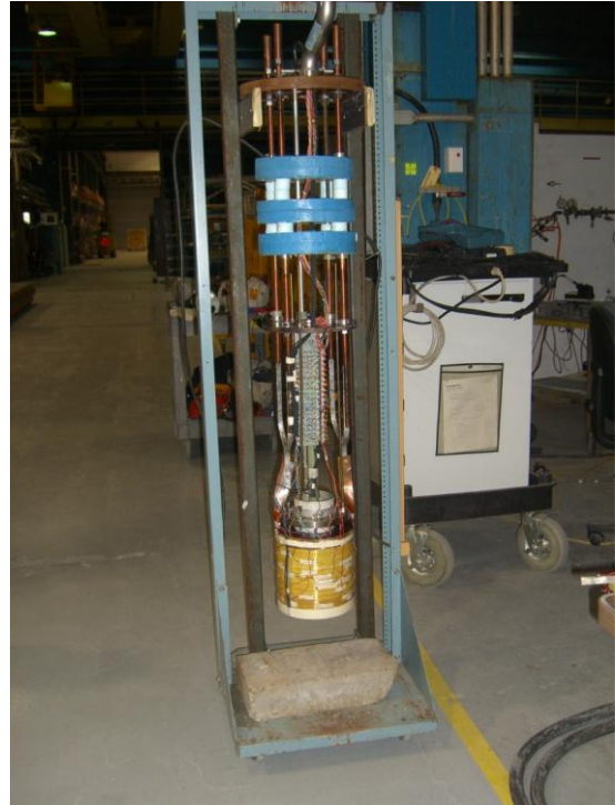
Fig. 10: Photographs of the coil on top-hat with all instrumentation while being prepared for 4 K test.
