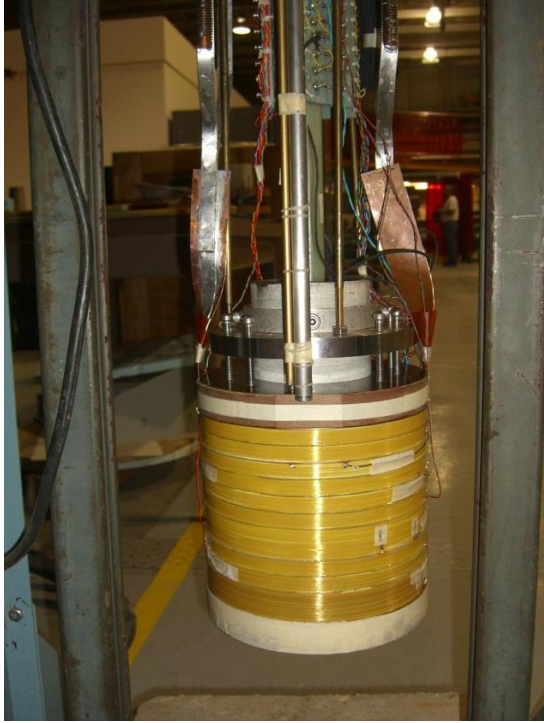
Fig. 10: Photographs of the coil on top-hat with all instrumentation while being prepared for 4 K test.
