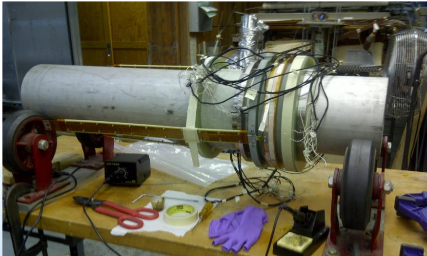
Each outer pancake uses ~200 m of conductor
