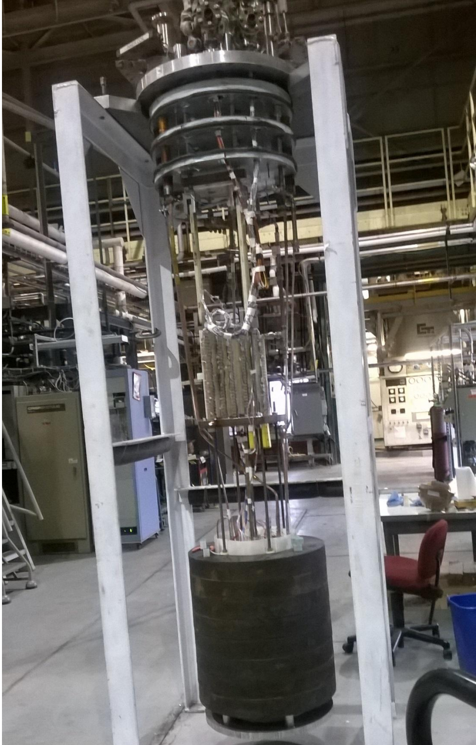
Figure 4: SMES coil installed on the top hat for testing.
