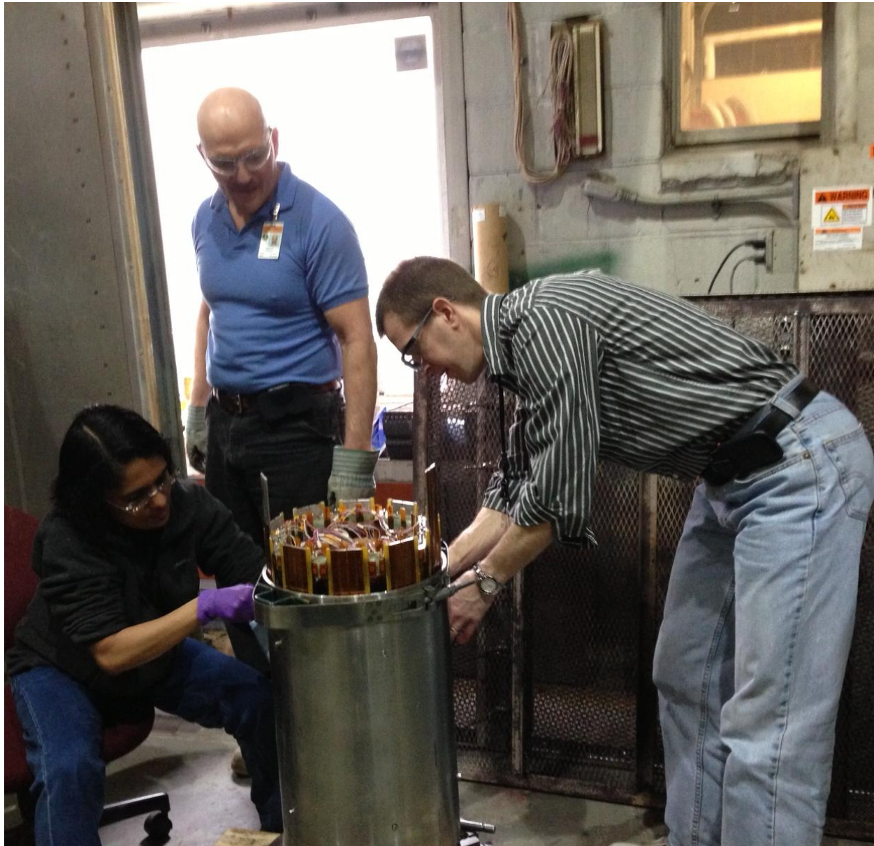
Figure 1: Outer coil with stainless steel support tube being installed.
