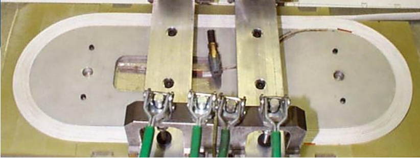
Magnet DCC006: 2 nd HTS Dipole (Magnet No. 6 in the common coil cable magnet series)
