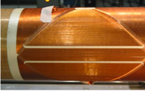
Fig. 2. A highly filled winding pattern of an optimum integral direct wind coil with midplane turns extending full length.
