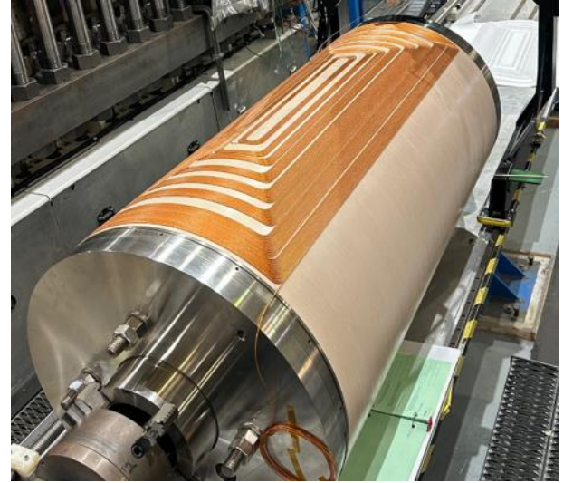
Fig. 9. First quadrant of the first layer of B0pF winding based on the separated function optimum integral design.
