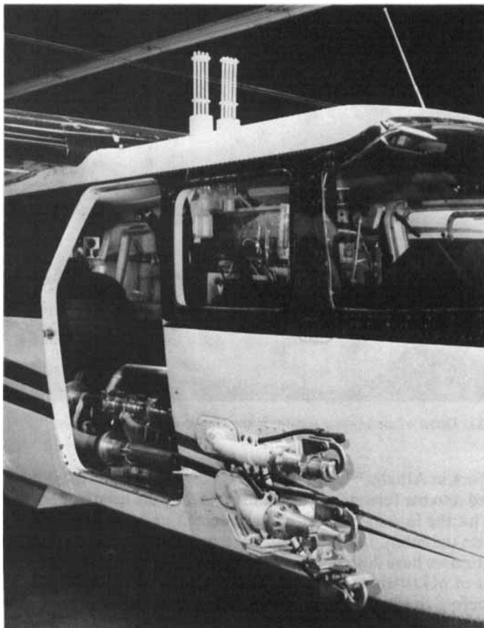
FIGURE 21. Detail of research aircraft showing inlets for air samples ( lower right , with remote-operated covers), cloudwater separator (in cabin), cloudwater collectors (protruding through cabin roof) and collection bottles (in cabin).
