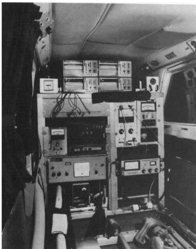
FIGURE 24. View of rear instrument rack in the aircraft, showing on the left , the data acquisition system, navigational instrument read-outs, Doppler radar, and the integrating-nephelometer. On the right are the chemiluminescence ozone monitor, the high-volume flowmeter and integrator, radiation thermometer and the turbulence monitor. Strip-chart recorders are on top of the rack.
