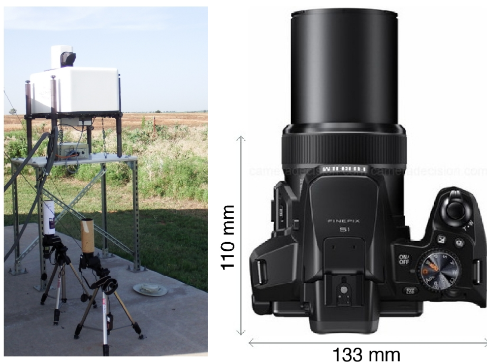
Figure S11. Left , deployment of cameras at ARM Southern Great Plains Site in north central Oklahoma. Tubes mounted on lenses prevent direct solar beam from hitting the lens. At rear is Doppler Lidar. Right , camera with zoom lens fully extended to 1200 mm 35-mm equivalent focal length (actual focal length 215 mm for the so-called 1/2.3-inch ( 6.17 \times 4.55 mm) sensor).
